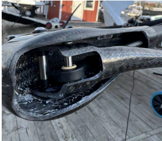
Figure 3.4. Wand attachment on a production Moth dinghy, as seen from below.
