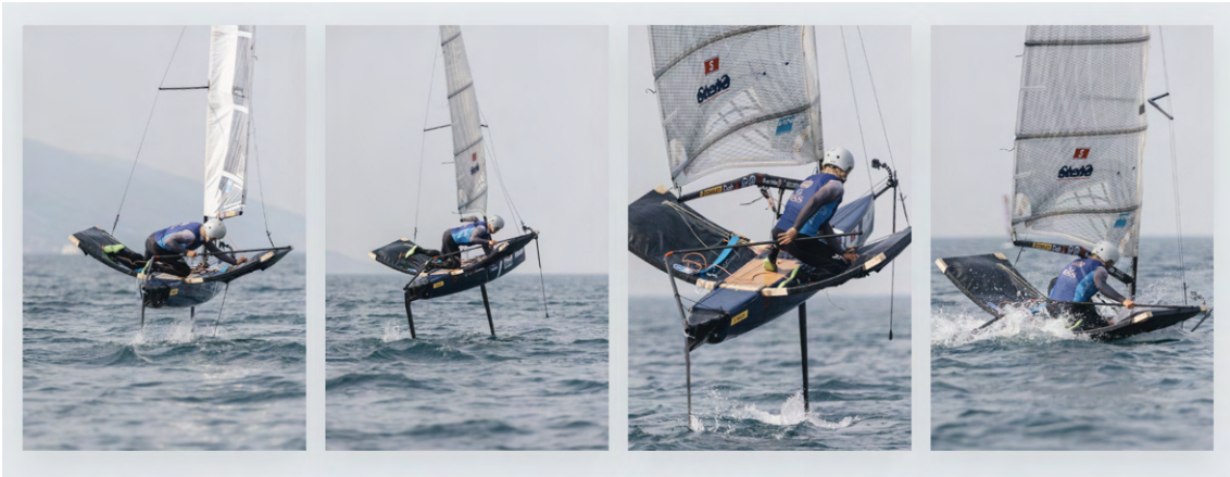
Figure 1.11. Illustration of foil-induced launch. The control system reacts to an incoming irregular wave by increasing foil lift, but as the wave passes and the water surface returns to normal, the excess lift launches the vessel clear of the water.
