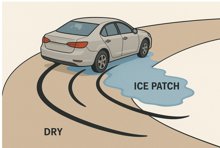
Figure 1.2: A vehicle entering a curve with a low-friction section, risking loss of control from insufficient speed adaptation.
