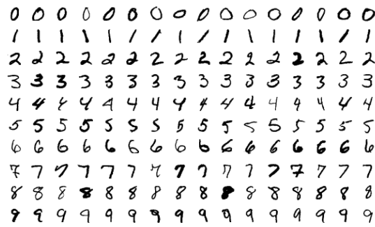
Figure 3.1: Example images from the MNIST dataset. Consisting of images with resolution 28x28, depicting handwritten digits in grayscale.
