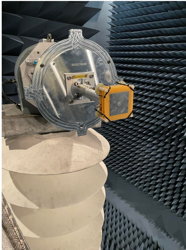
Figure 7.7: Antenna mounted in the anechoic chamber.
