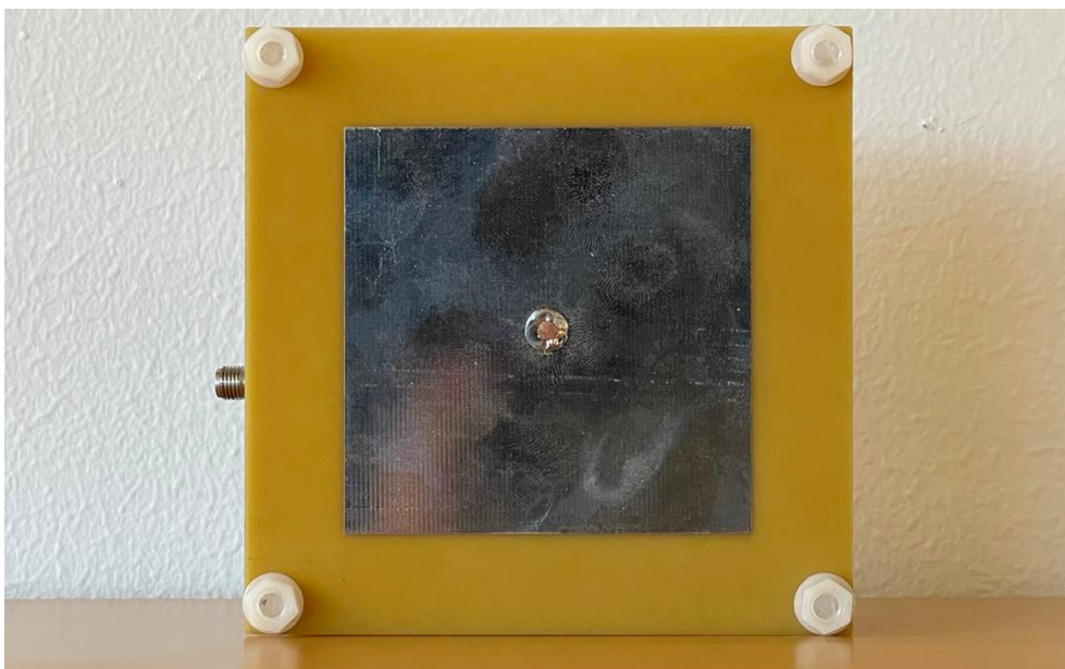
Figure 6.8: Assembled antenna top view
