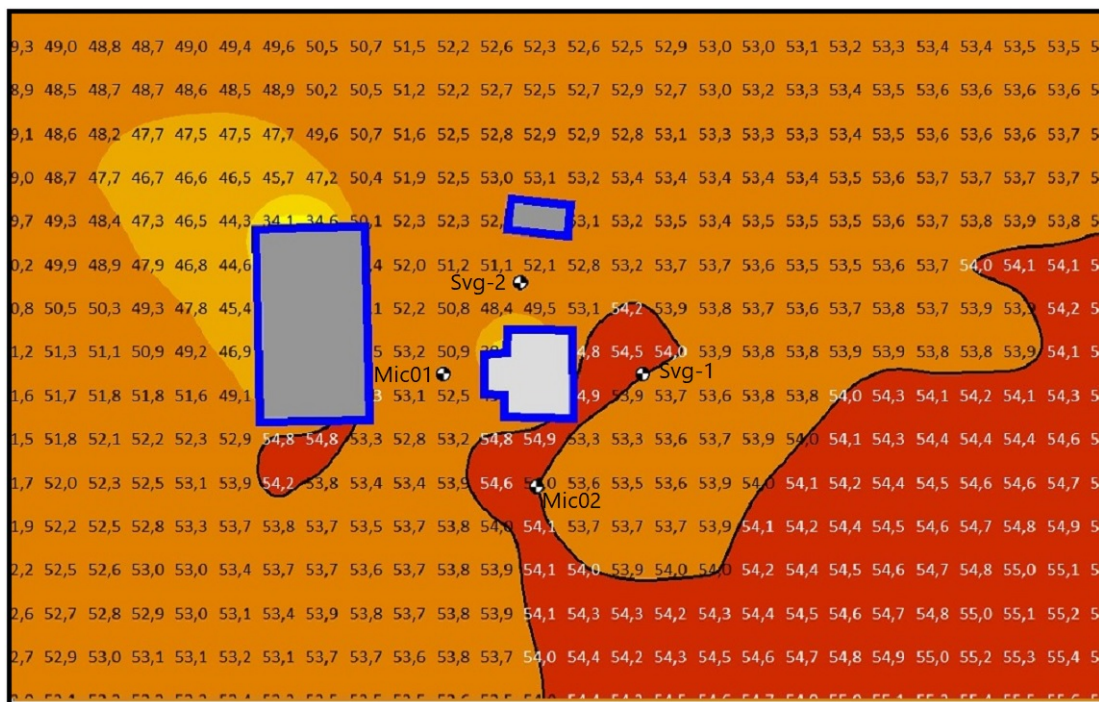
Figure B.13: Grid Noise Map based on Nord2000 for the noise indicator L_{den} in the winter at Lånheveien 11.
