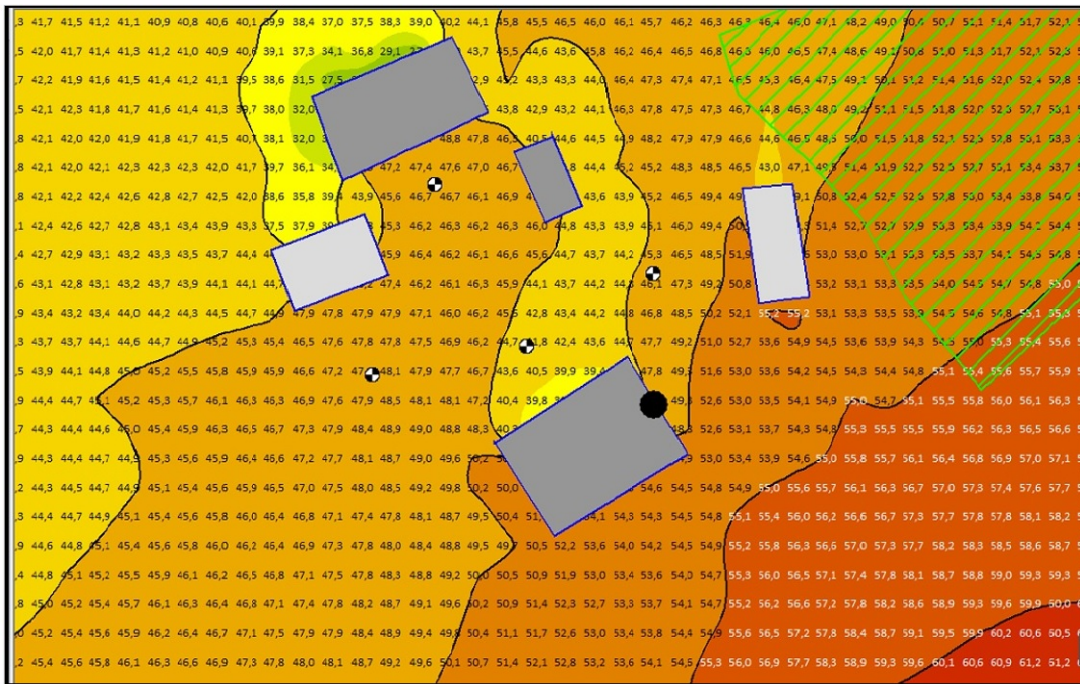
Figure B.2: Grid Noise Map based on Nord2000 for the noise indicator L_d at Solbergveien 37 in the winter.
