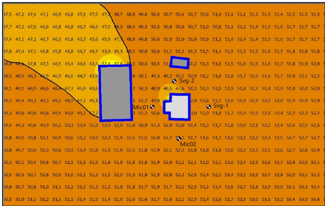
Figure B.14: Grid Noise Map based on Nord2000 for the noise indicator L_d in the winter at Lånheveien 11.
