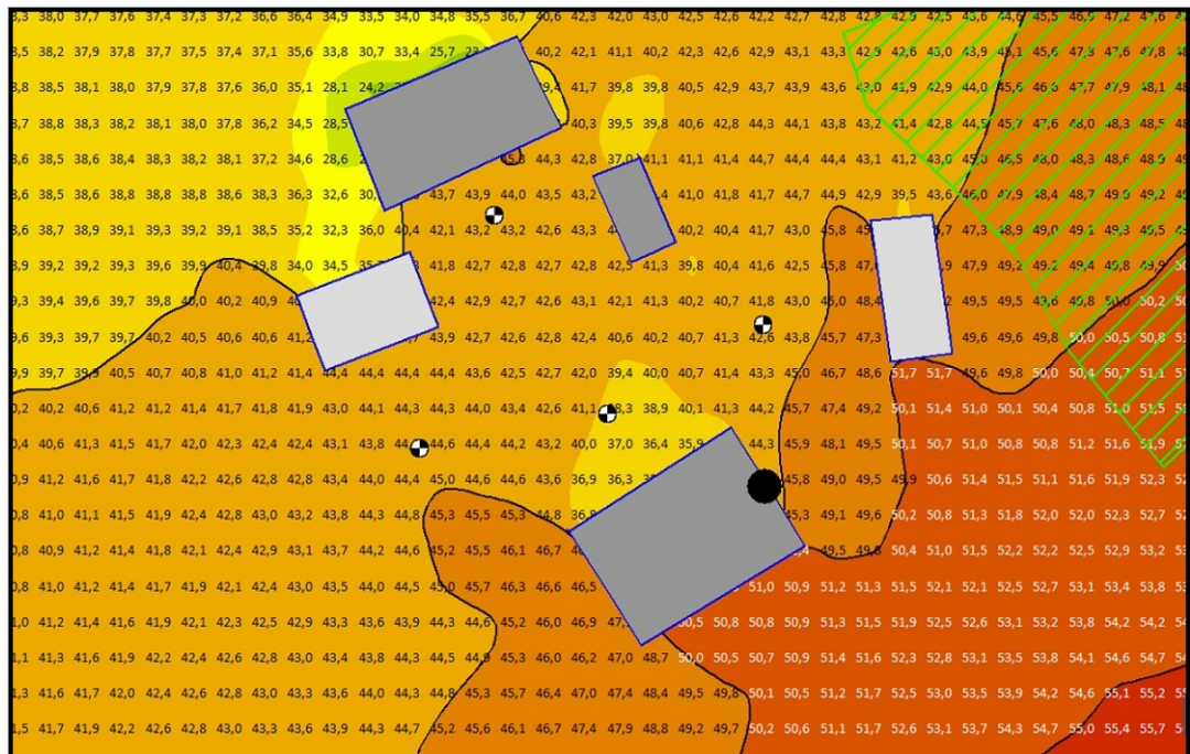
Figure B.3: Grid Noise Map based on Nord2000 for the noise indicator L_e at Solbergveien 37 in the winter.
