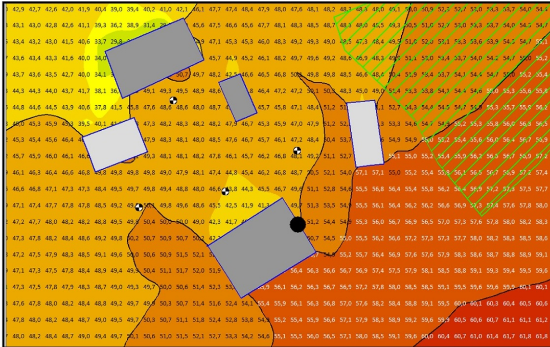
Figure B.1: Grid Noise Map based on Nord2000 for the noise indicator L_{den} at Solbergveien 37 in the winter.
