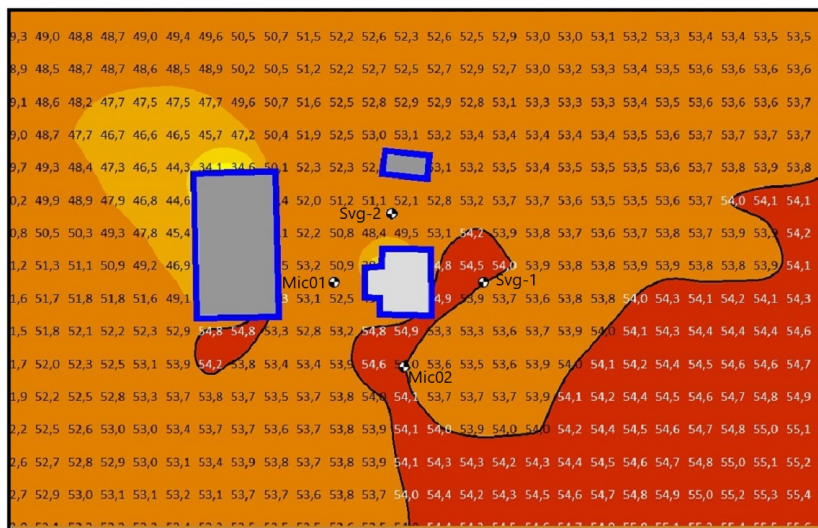
Figure 5.21: GNM and the predicted noise levels based on Nord2000 for the noise indicator L_{den} in the winter at Lånheveien 11.
