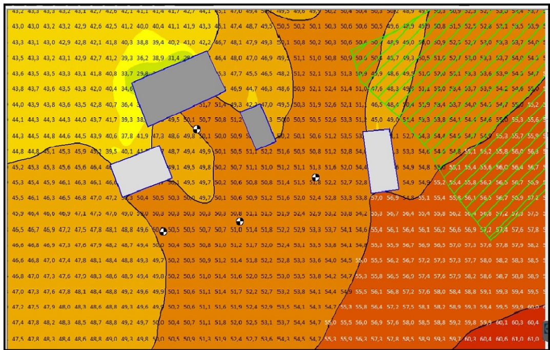
Figure B.9: Grid Noise Map based on Nord2000 for the noise indicator L_{den} without the building near to E18 at Solbergveien 37.
