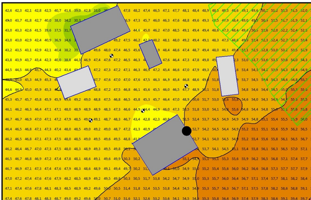
Figure B.5: Grid Noise Map based on Nord2000 for the noise indicator L_{den} at Solbergveien 37 in the summer.
