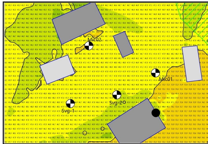
Figure 5.3: Grid Noise maps (GNM) and the predicted noise levels based on RLS-90.
