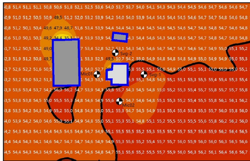
Figure 5.20: GNM and the predicted noise levels based on Nord2000 for the noise indicator L_{den} in the summer at Lånheveien 11.
