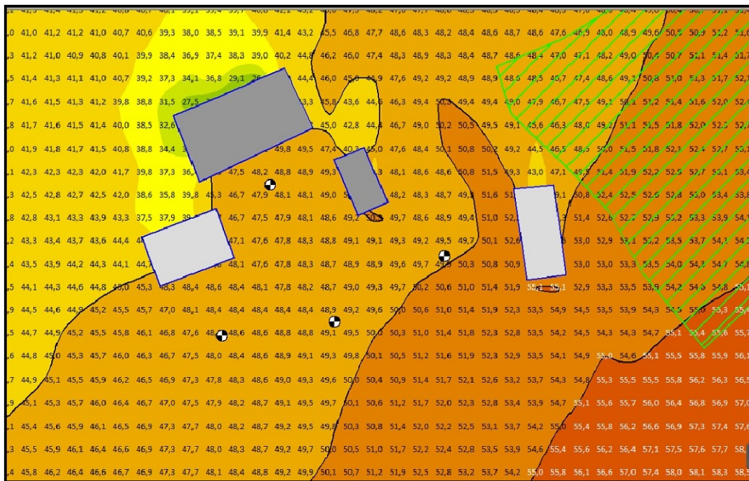
Figure B.10: Grid Noise Map based on Nord2000 for the noise indicator L_d without the building near to E18 at Solbergveien 37.
