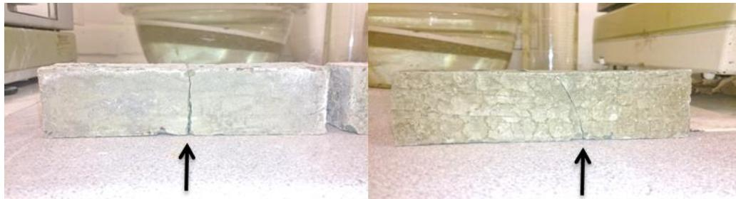
Figure 15. Fracture pattern of stabilised sediment; C1 (left) and C2 (right).
