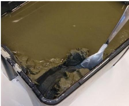
Figure 9. Sampled sediment. Notice the difference in colour between oxidised surface and underlying sediment.
