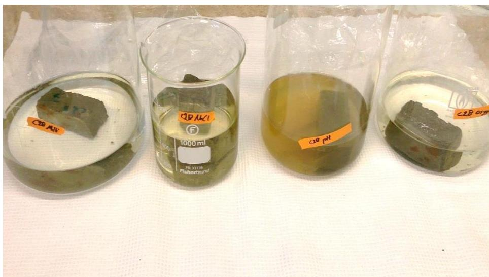
Figure 20. Leachate from stabilised sediment C2B. From left to right: Milli-Q, NaCl, pH and Oxygen
