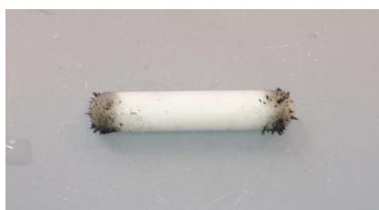
Figure 11. Flakes of metal attached to a magnet flea.
