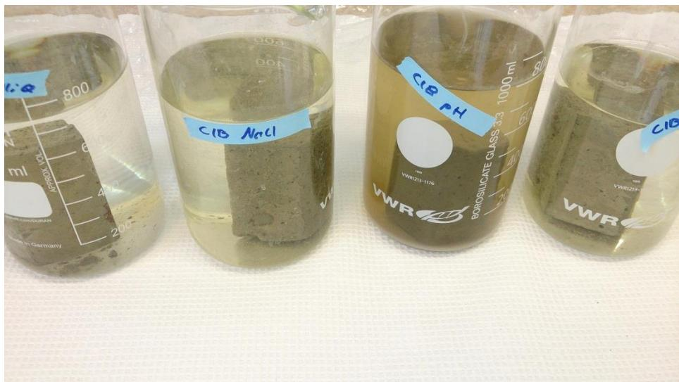
Figure 19. Leachate from stabilised sediment C1B. From left to right: Milli-Q, NaCl, pH and Oxygen.
