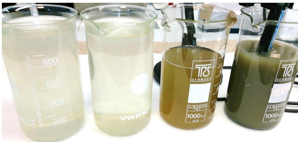
Figure 18. Leachate from sediment surface diffusion test. From left to right: Milli-Q, NaCl, pH and Oxygen.
