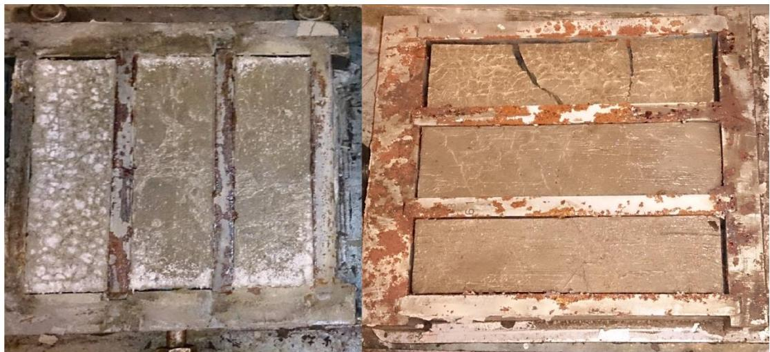
Figure 14. Stabilised sediment on the 18<sup>th</sup> day of curing; C1 (left) and C2 (right).
