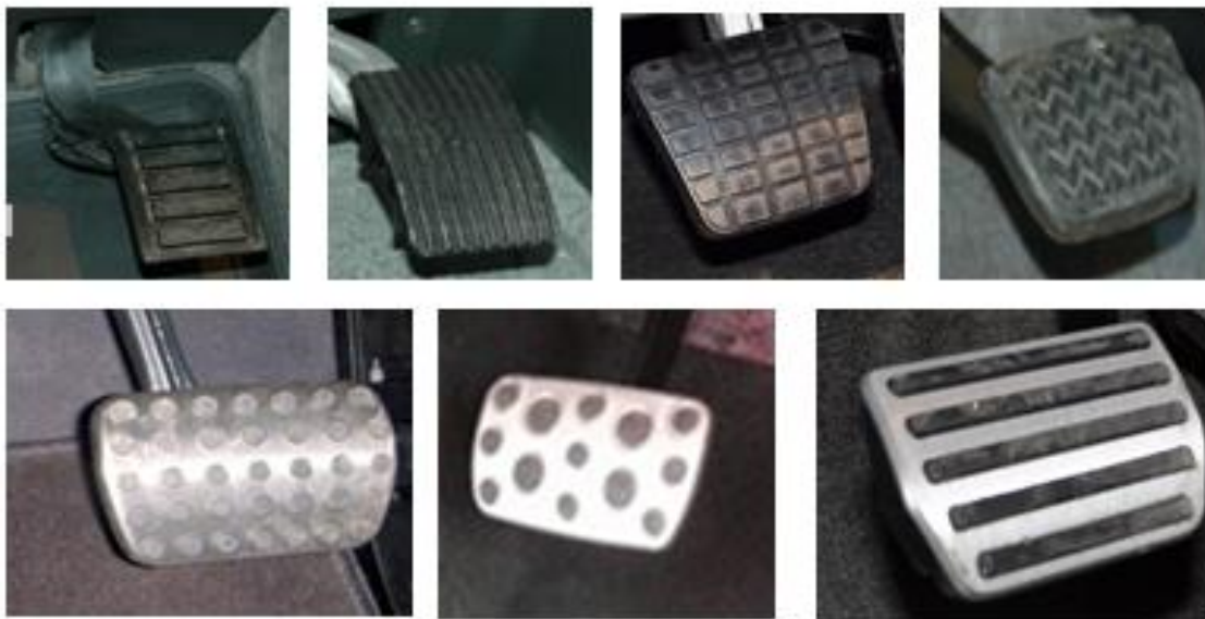
Figure 50 Pedal friction Patterns
