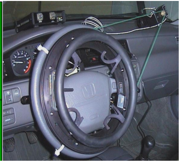
Figure 22 Measuring steering wheel adaptor
