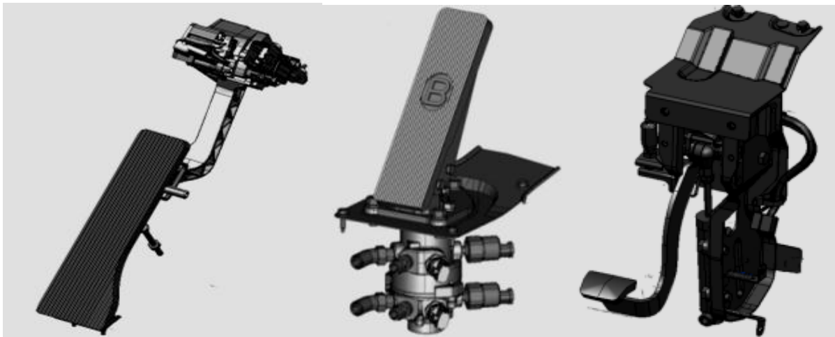
Figure 41 combination of floor mounted and suspended pedals
