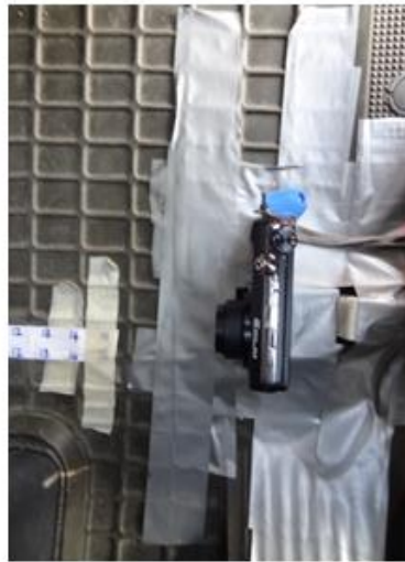
Camera 1 being attached with Mounting Fixture 1
