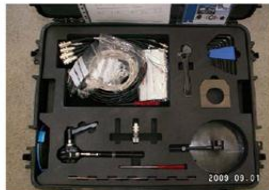
Figure 28 Ricardo Gear Shift Quality Assessment (GSQA) installations
