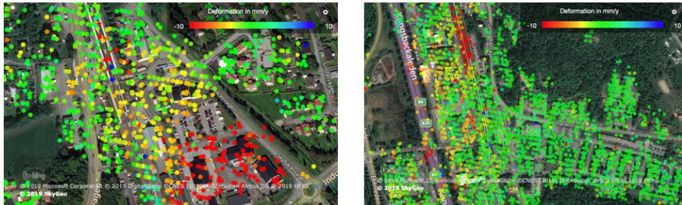
**Figure 4.18:** Displacement maps over Lindome station (Left) and Källered station (Right) using Sentinel-1 data processed by SkyGeo. Note that the dots do not represent the pixel size, they show the center of the pixel. The images are courtesy of SkyGeo and used with permission from SkyGeo, WSP and Trafikverket. The data is shown in a map by Bing.
