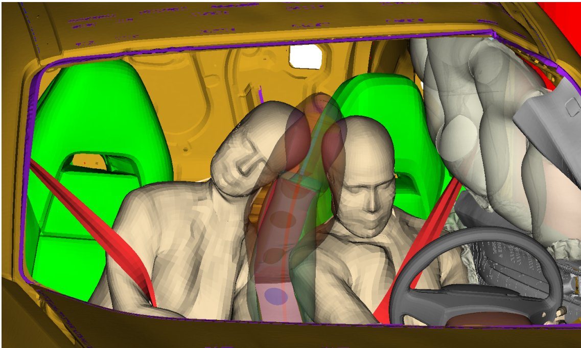
Figure H.2: A snapshot at 102 ms of the minimum Head2Head distance in configuration C3-E
