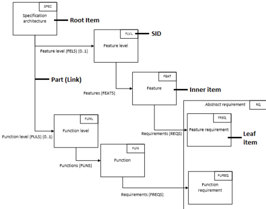
Figure 2.1: Example of a requirement meta model in SystemWeaver
