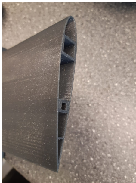
Figure 5.8: Hollow section of the bottom strut ending close to the wing
