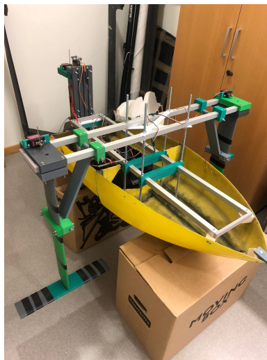
Figure 3.25: Workshop inclining test setup
