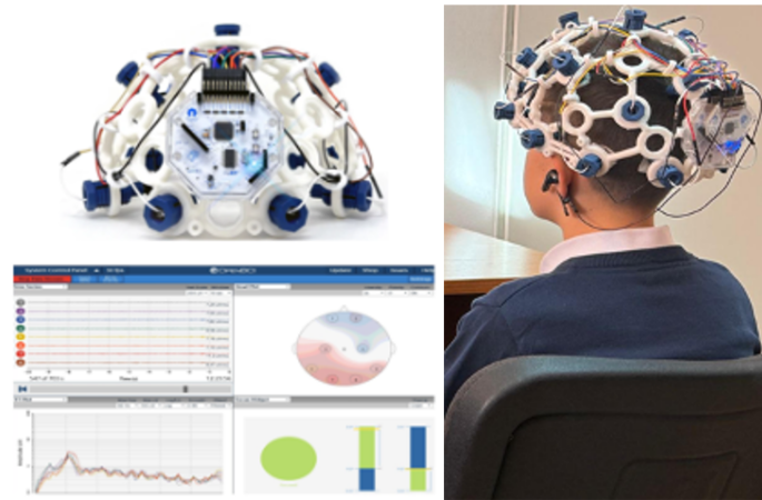
Figure 3.1: EEG recording setup showing the Ultracortex Mark IV headset with 16 dry electrodes and the OpenBCI CytonDaisy acquisition system.
