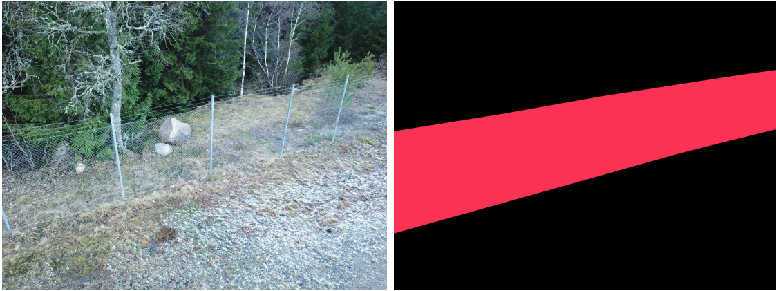
Figure 5.3: Side view image of a fence and its mask. The mask is the ground truth and shows the neural network what to classify. The mask has two classes, the background in black and the fence classified in red.
