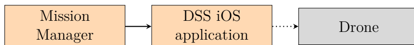
Figure 4.5: High-level view of the communication between the Mission Manager and DSS application and subsequently the drone.
