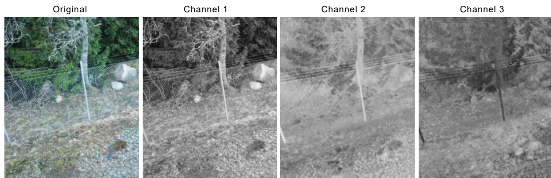
Figure 5.8: Showing the original image split up into different channels, which shows how different channels can highlight different features in the image.
