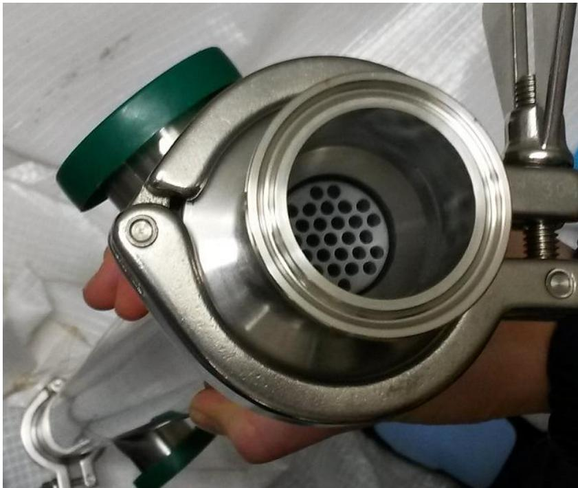
*Figure C3. The membrane right before installed in the pilot plant.*
