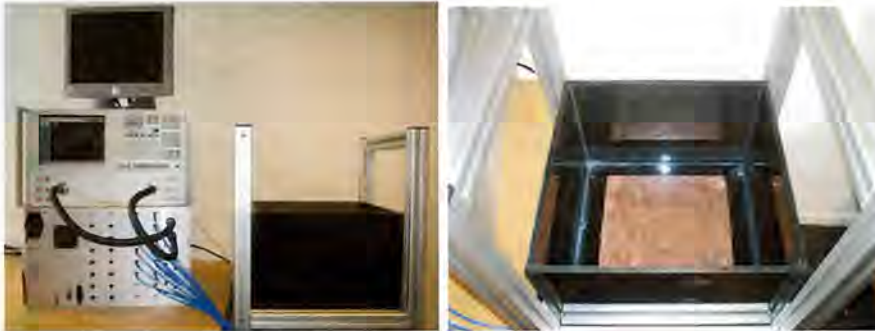
Figure 1.2: The experimental prototype at Chalmers. A network analyzer connected to an antenna array.
