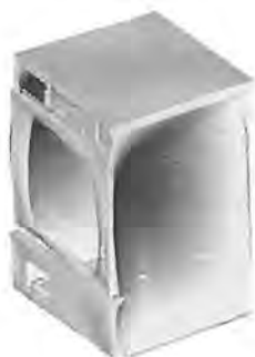
Figure G3: Mode 3 of entire washing machine.
