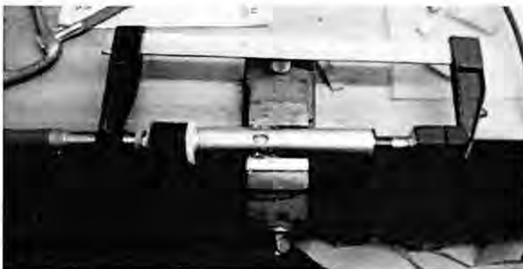
Figure 3-3: Compressed spring leg during removal of damping foam.
