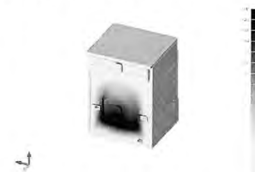
Figure F2: Mode 2 of the steel shell.
