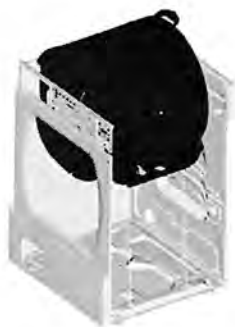
Figure G1: Mode 1 of entire washing machine.
