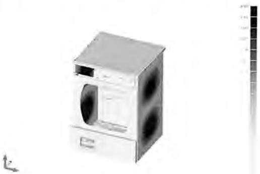
Figure F5: Mode 5 of the steel shell.
