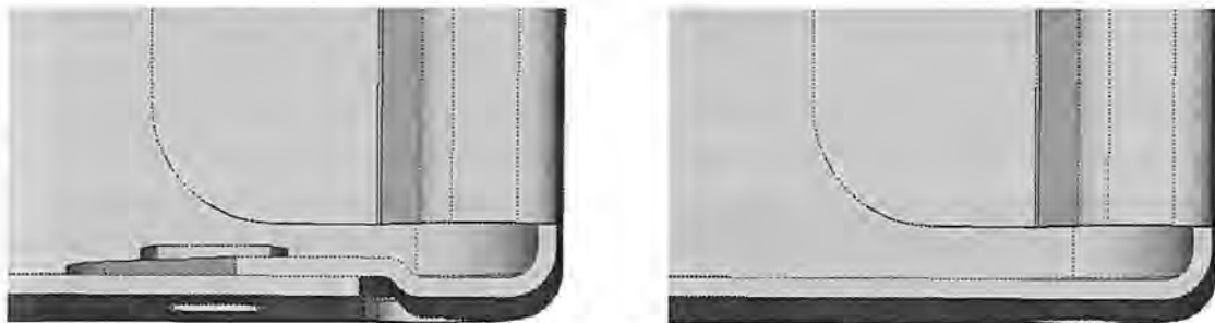
Figure 3-1: Original geometry to the left and simplified geometry to the right.
