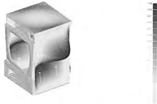
Figure G10: Mode 10 of entire washing machine.
