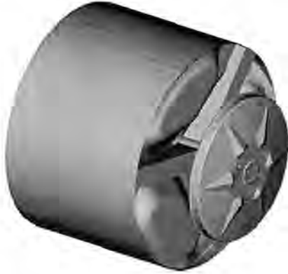
Figure 2-16: FE-model of the rotating inside parts, belt pulley, convey and axle, drum back piece and drum.
