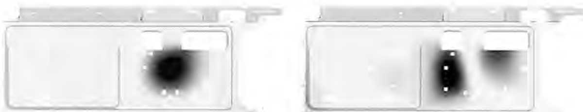
Figure 5-13: Iso surfaces showing the mode shape of the electric bridge. Mode four to the left and mode six to the right.
