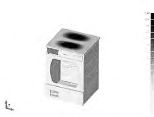
Figure F8: Mode 8 of the steel shell.
