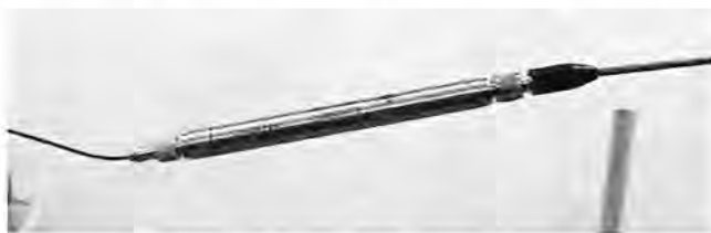
Figure 2-12: Charge-to-Deltatron converter for the load cell signal.
