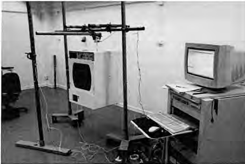
Figure 2-9: A complete experimental setup where the washing machine shell is fitted with accelerometers. Visible in the figure are the washing machine, shaker, accelerometers, amplifier, VXI and computer.
