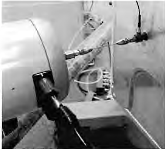
Figure 2-11: The Shaker, stinger and load cell.
