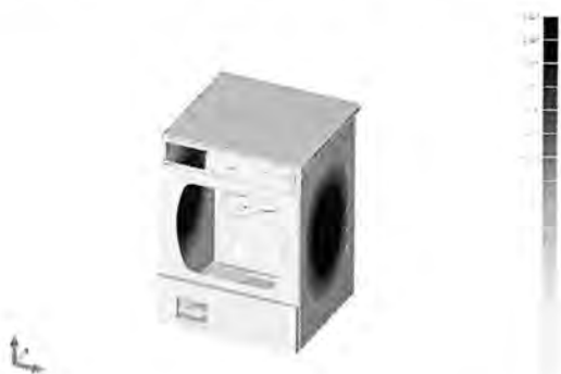
Figure F3: Mode 3 of the steel shell.
