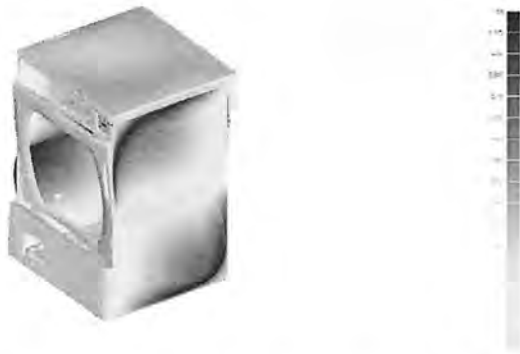
Figure G9: Mode 9 of entire washing machine.
