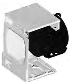
Figure G1: Mode 1 of entire washing machine.
