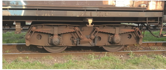
Figure 2.5: Bogie with leaf springs. Figure by the authors.
