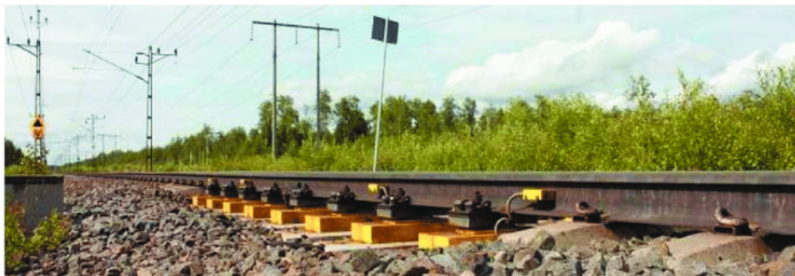
Figure 3.5: Wheel impact load detector at Sunderbyn. Figure by Matthias Asplund, Trafikverket, from [29].
