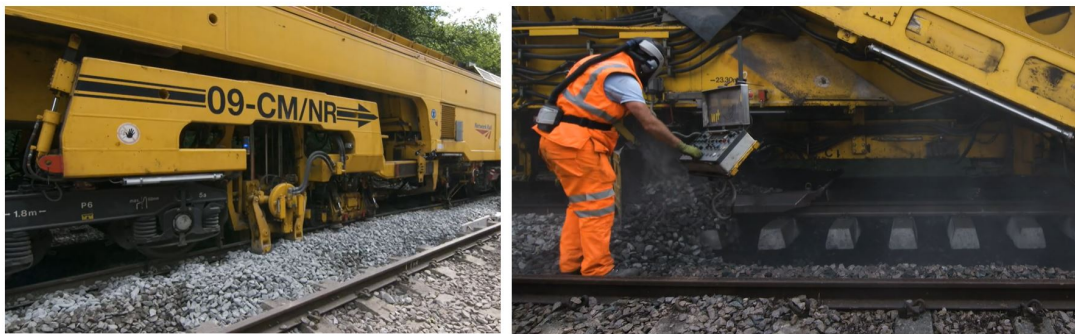
Figure 3.3: Tamper and ballast regulator. Figure from [26].
