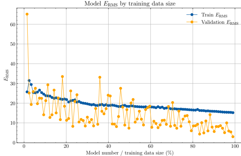
Figure 4.3: This figure presents the E_{RMS} of the model as the training data size ranges from \approx 1\% to \approx 99\% . The method explained in Section 3.6 was applied and the time range of the data is [1.1.2023, 1.4.2025]. Both train E_{RMS} (blue) and validation E_{RMS} (orange) decrease with increasing data size, with the slope becoming more gradual as the data size approaches 100%. The curves reflect a downward trend in E_{RMS} as more data is incorporated.
