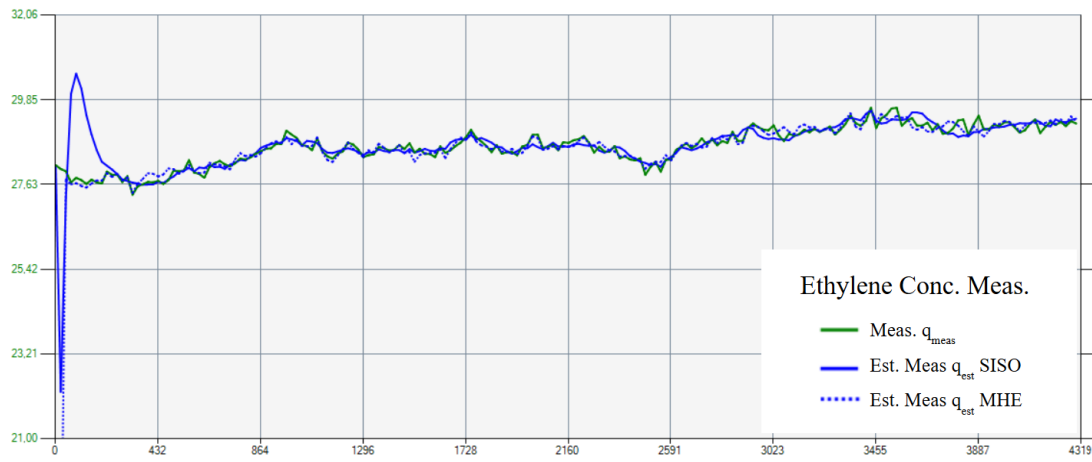
(a) The true and estimated measurements of ethylene concentration in mol% with SISO and MHE.
