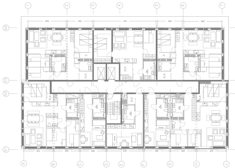
Figure 4.7: Typical apartment floor plan of Building C.
