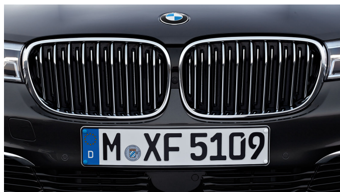
Figure 7.4: Kidney grille integrated with an AS on BMW Serie 7 (BMW, 2015)
