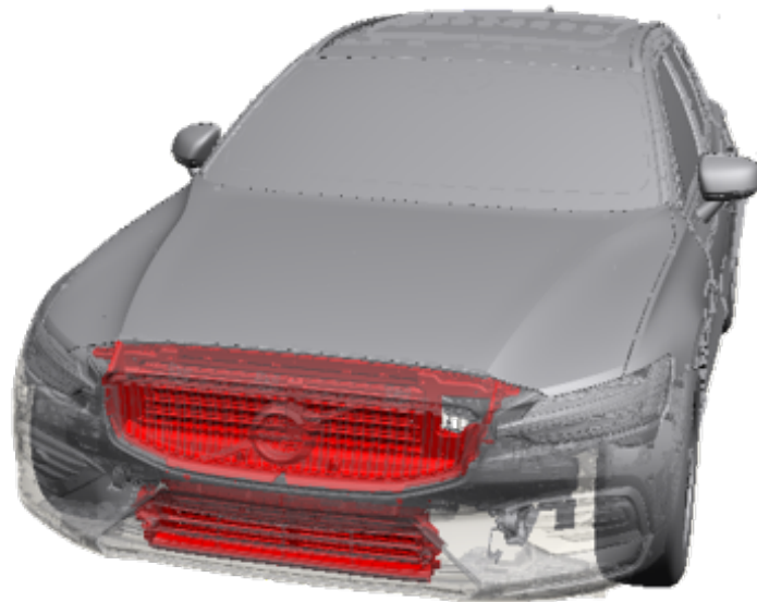
Figure 2.1: CrossSection of the Front of a vehicle, where the active shutter systems are marked in red
