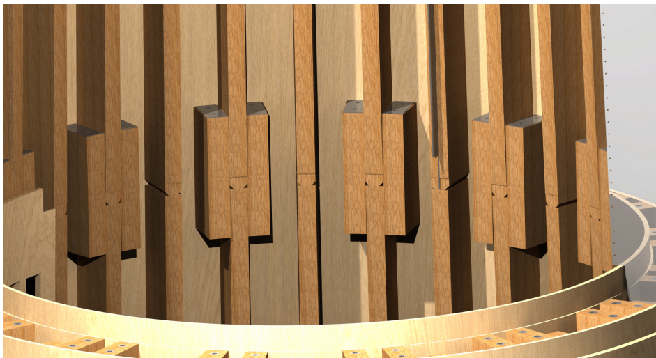
Figure 25: Vertical joint at the top
