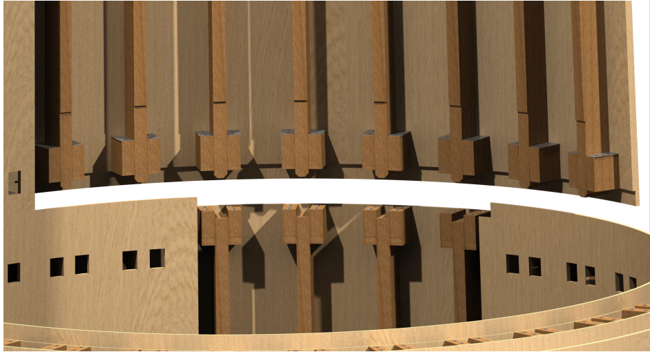
Figure 24: Removed LVL, shows stacking
