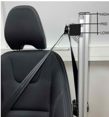
(a) B-pillar installation (mid position), with high and low positions indicated ( 25^\circ upright seatback).
