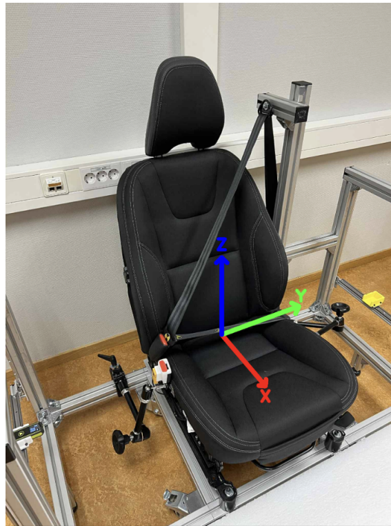
Figure 3.1: The test rig consisting of a front car seat mounted in a rigid steel frame, with X, Y, and Z coordinate directions relative to the rig.
