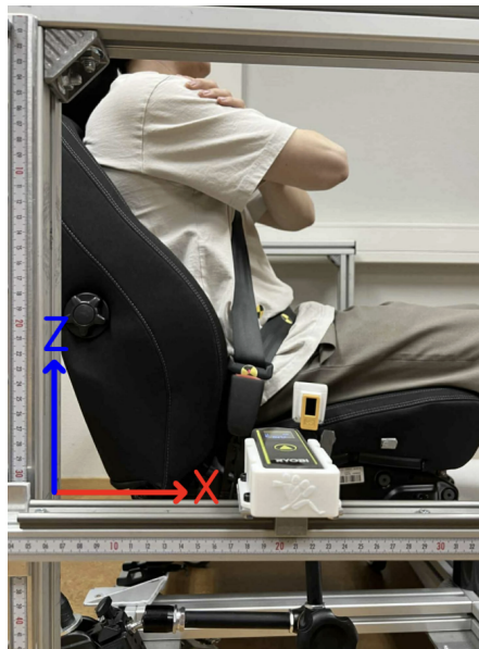
Figure 3.5: The laser measurement system consists of a movable laser that determines the depth (y-axis) and integrated rulers placed on the frame that captures the x- and z-coordinates). The figure shows the measurement of the buckle position.
