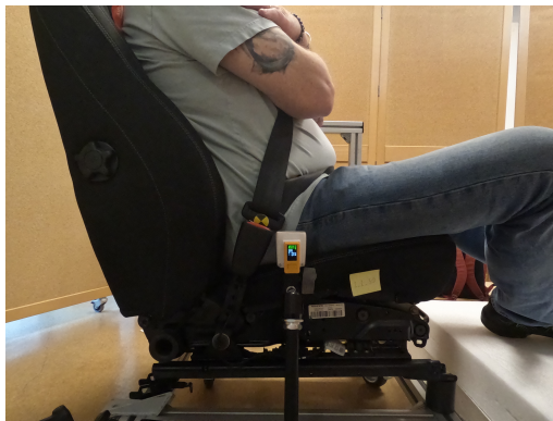
Figure 4.4: Example of lap belt folding associated with an abdominal fold during testing (participant ID 30).
