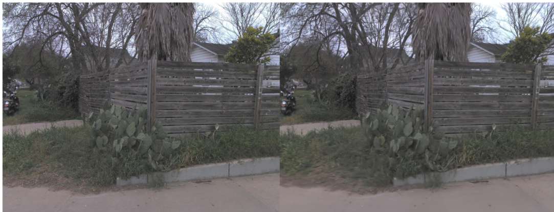
Figure 2.13: Comparison between a ground-truth image and the corresponding 3DGS reconstruction. Left: ground-truth image. Right: reconstruction showing grainy artifacts in the grass region.
