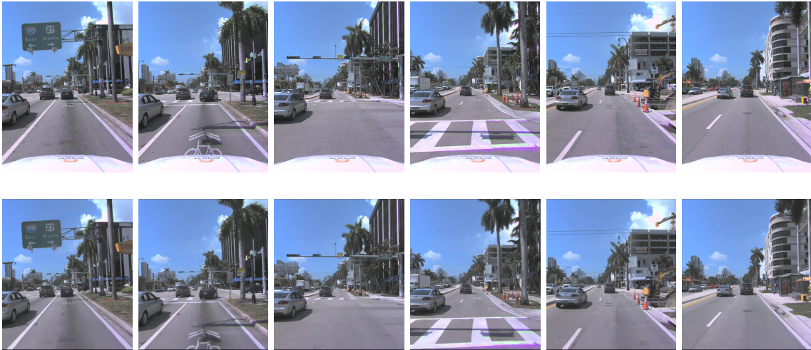
Figure 4.1: Top row: original logged frames. Bottom row: corresponding SplatAD renders from similar poses.
