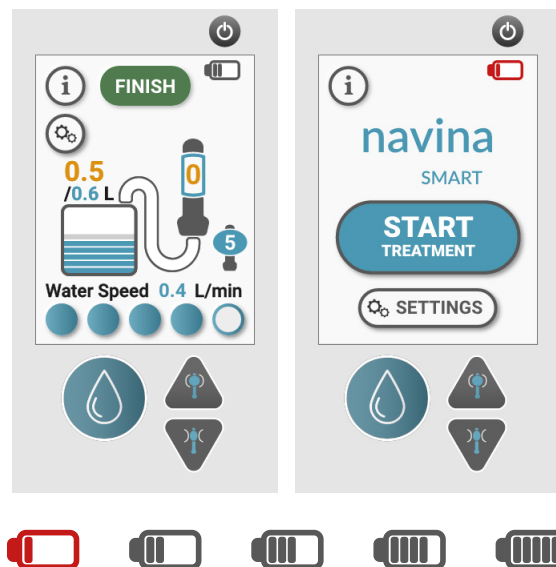
Figure 39: the prototype showing how the battery bar can look with varying amounts of battery left.
