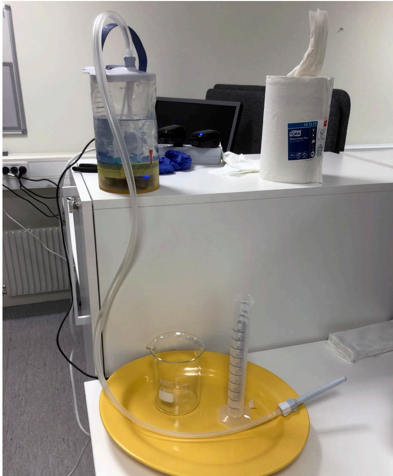
Figure 22: the pump station prototype pumping water and air to the catheter.
