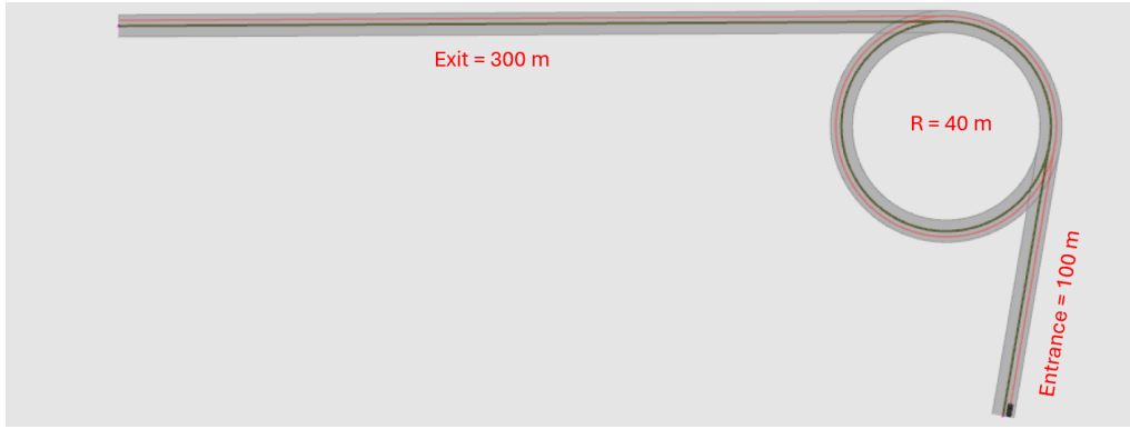
Figure 4.5: Driving scenario used in CarMaker simulation.
