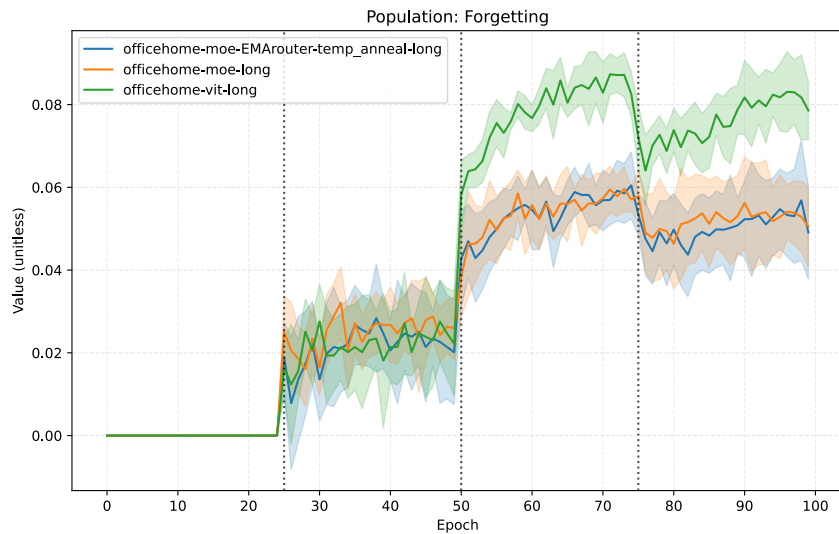
Figure 4.15: Forgetting measure for long training time on Office-Home dataset. The MoE models forget significantly less than the dense variant as more domains are presented.
