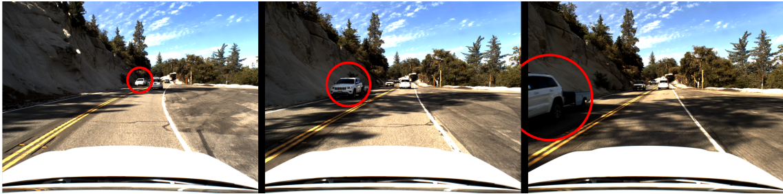
Figure 7.12: Three camera frames showing the oncoming target vehicle encircled in red. In the rightmost frame it can be seen that the vehicle is towing a trailer.
