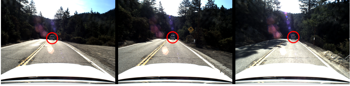
Figure 7.2: Camera frames of the following scenario covering the period during which the LIDAR gives faulty readings. Target vehicle is encircled in red.
