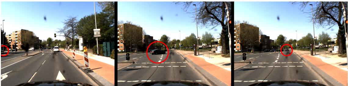
Figure 7.21: Frame sequence shows the car as it is discovered by the sensors, enters the intersection and starts heading down the road
