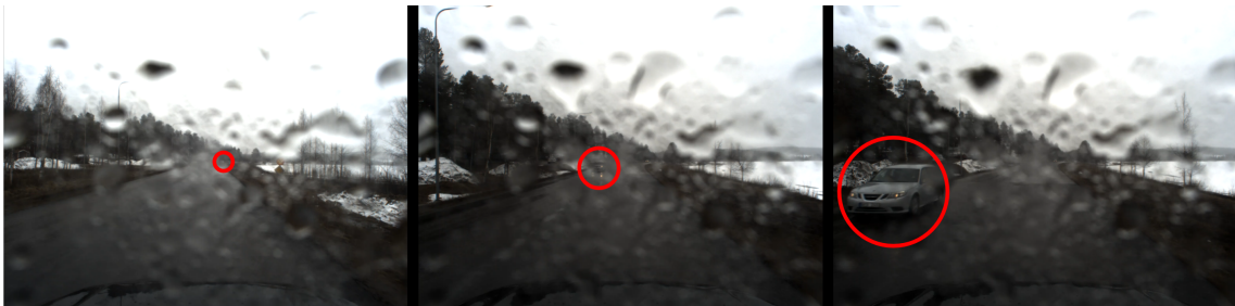
Figure 7.17: Three frames showing the oncoming vehicle encircled in red. The water obscures the oncoming vehicle in the first two frames
