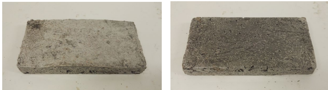
Test #1.2: Concrete casting with 60% concrete and 40% slag-stones (size 2-10 mm)
