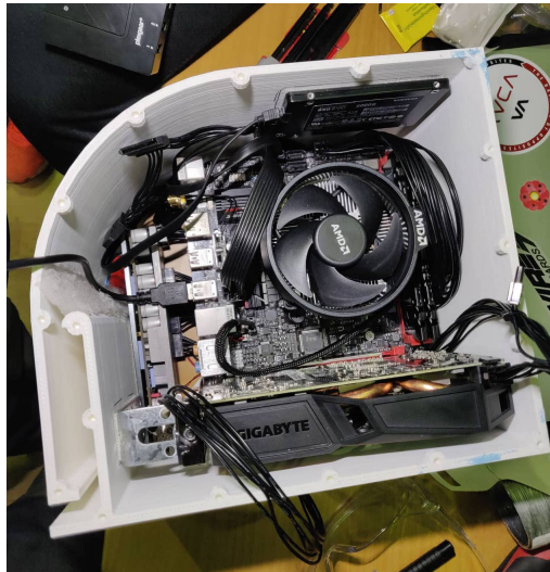
Fig. 4.6. The final product with all components mounted (without sides).
