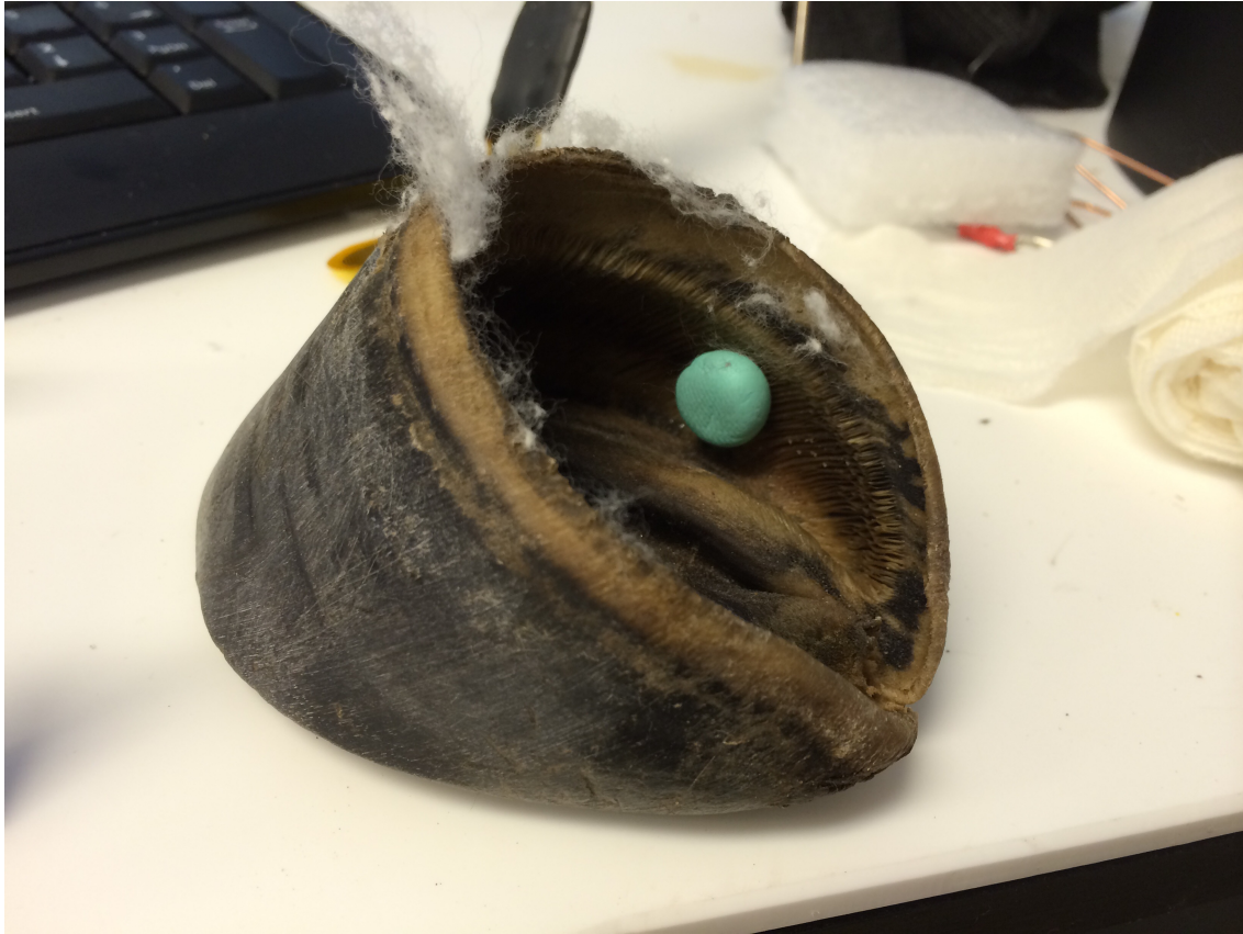
Figure 2.5: The blu-tack is attached to the inside of the hoof to mimic a keratoma.
