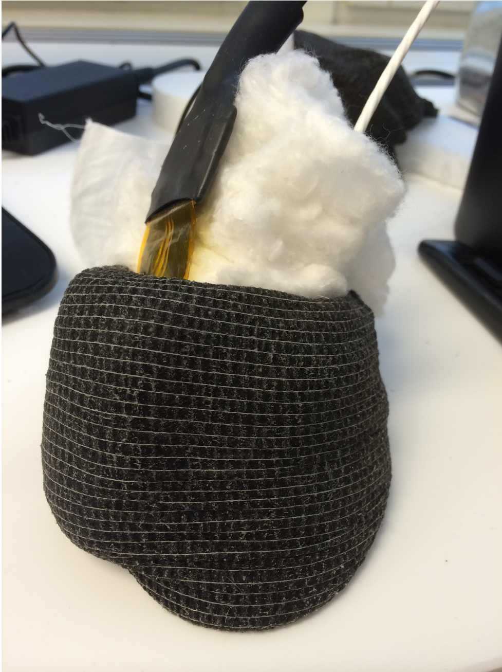
Figure 2.2: Experimental setup with the sensor attached to the hoof with vetflex. The hoof is then filled with cotton to get an insulating background and to prevent air flow inside the hoof. The white cable is the reference temperature sensor and the black cable is the sensor taking the measurement.
