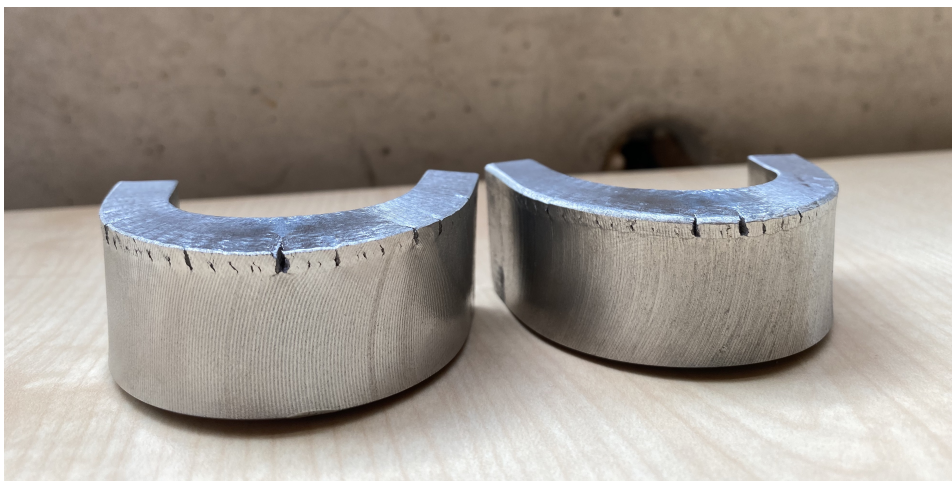
Figure 4.2: Results from the performed bend test on two test samples, indicating the adhesion between cladding and substrate.
