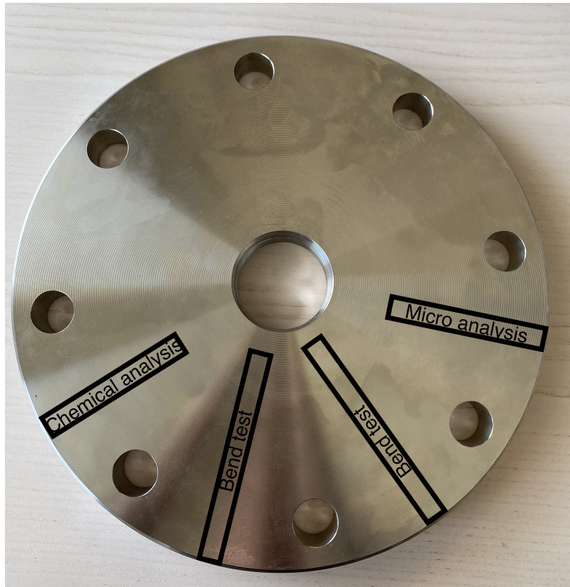
Figure A.1: Schematic of sample cut from clad flange
