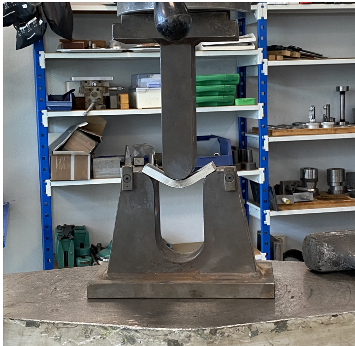
Figure 3.4: Procedure of three point side bend test.
