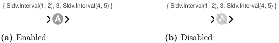
Figure 5.3: SLDV Assumption block. The block lets SLDV assume the input signal is in the set \{[1, 2], 3, [4, 5]\} .
