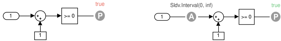
(a) Model without Assumption block, falsified by SLDV. (b) Model with Assumption block, proven valid by SLDV.
