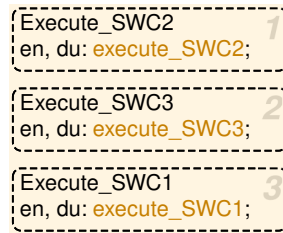
Figure 6.29: Changed Scheduler chart from Figure 3.1b to allow execution of SWCs in the very first time-step of the simulation.
