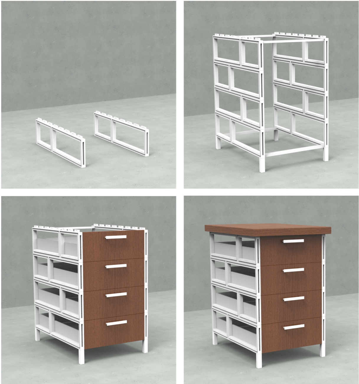
Figure 36. Assembling a storage module.
