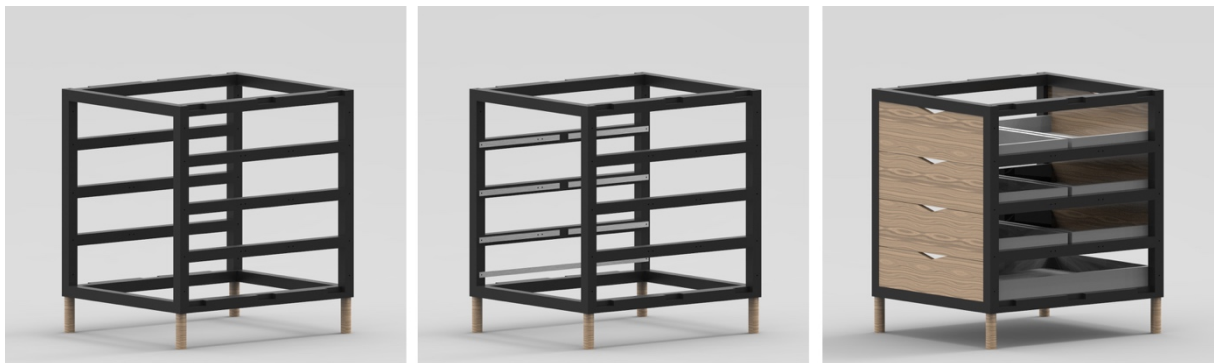
Figure 32. Idea to assemble the modules.
