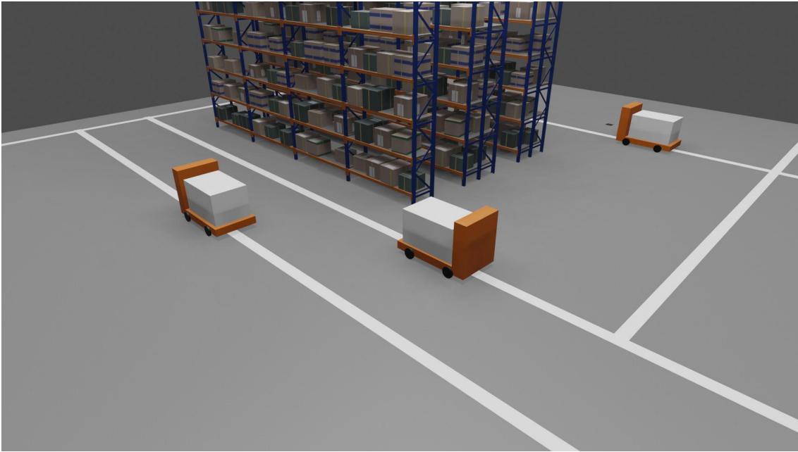
Figure 2.2: Visualization of rigid track guidance for AGVs
