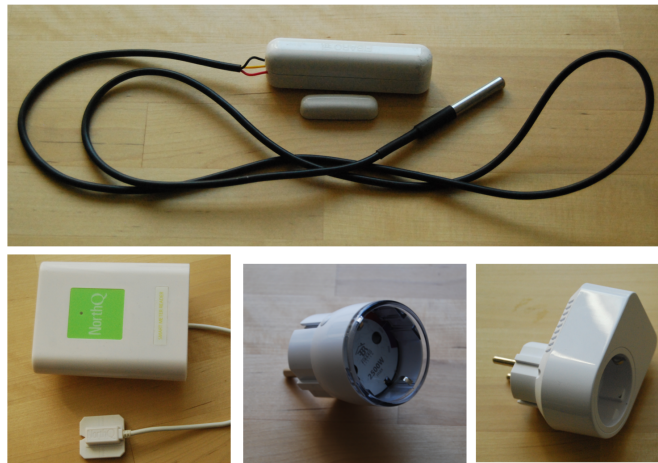
Figure 4.6: The Z-Wave sensors, Top: Fibaro Door/Window Sensor and DS18B20 Digital Thermometer, bottom left: NorthQ Power Reader, bottom middle: Fibaro System Wall Plug, bottom right: Energy Meter Aeon Labs ZW075-C16.
