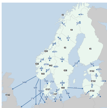
Figure B.2: Power Flow of the Nordic Power System - Winter Day [73]
