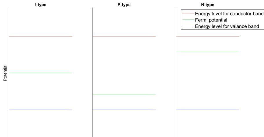
**Figure 2.4:** Band diagrams for semiconductors of i-, n- and p-type.
