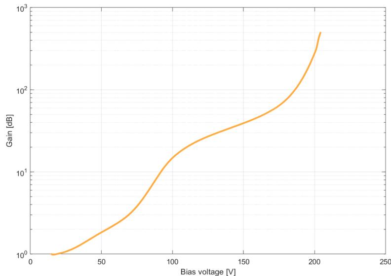
**Figure 2.8:** The gain as a function of bias voltage for an APD.
