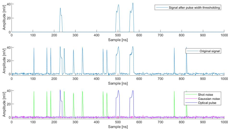
**Figure 4.5:** Signal after pulse width thresholding, original signal and its different segments.
