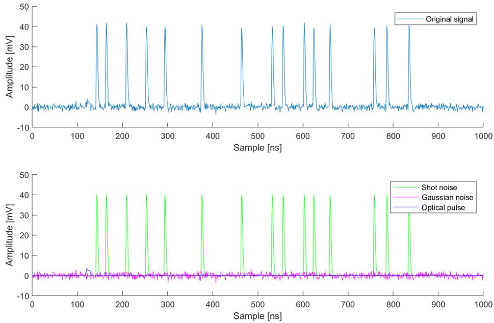
**Figure 5.2:** A typical signal in test case 2 and its different segments.
