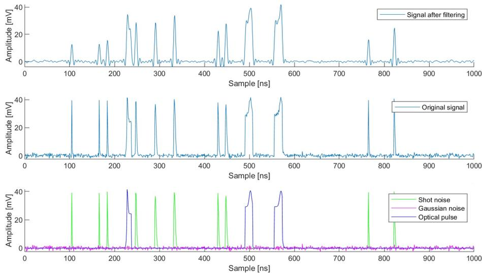
**Figure 4.3:** Signal after filtering, original signal and its different segments.
