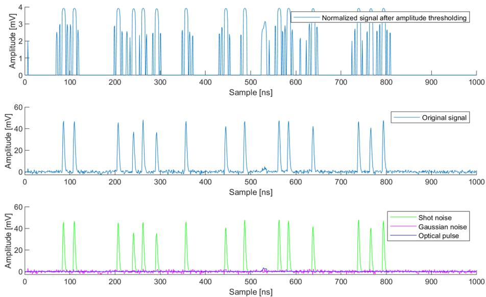
**Figure B.2:** Signal after normalizing, original signal and its different segments.
