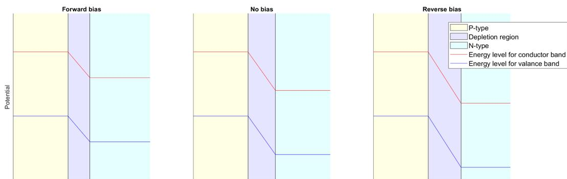
**Figure 2.6:** Band diagrams for three PN-junctions with different bias voltages; forward bias, no bias, reverse bias.
