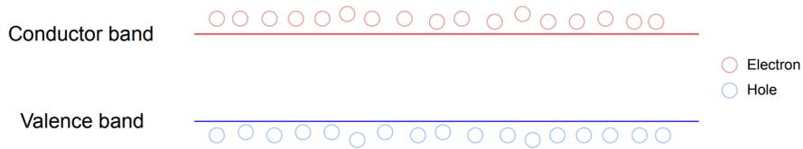
**Figure 2.3:** Band diagram for a typical semiconductor, the figure also illustrates the principle placement of electrons and holes.
