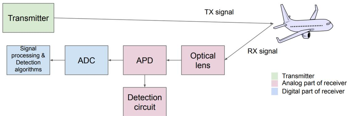
**Figure 2.1:** Simplified block diagram of the laser rangefinder principle.
