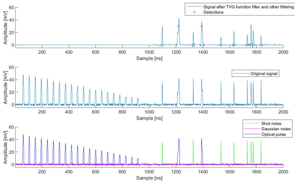
**Figure 5.9:** A signal after using the binary TVG function filter, the original signal and its different segments.
