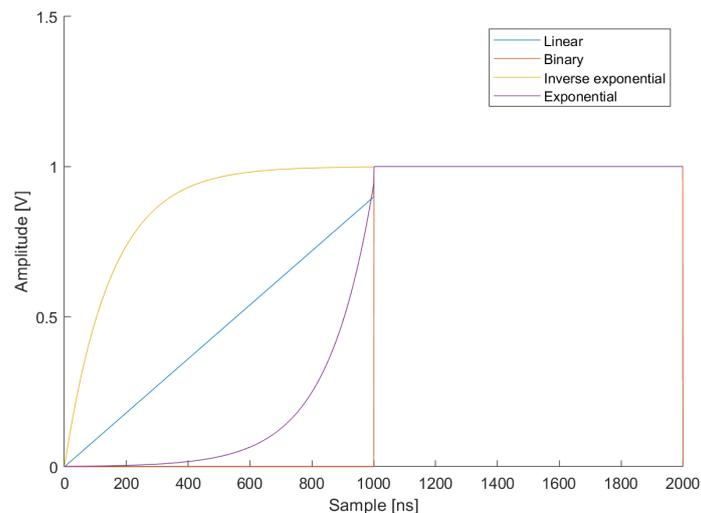
**Figure 4.6:** The four function filters investigated to replace the analog TVG.
