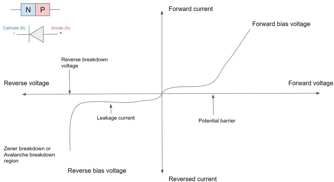
**Figure 2.7:** The IV-characteristics for a PN-junction. The leakage current is the same thing as dark noise current for an APD.
