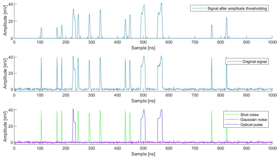
**Figure 4.4:** Signal after amplitude thresholding, original signal and its different segments.
