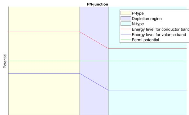
**Figure 2.5:** Band diagram for a typical PN-junction.
