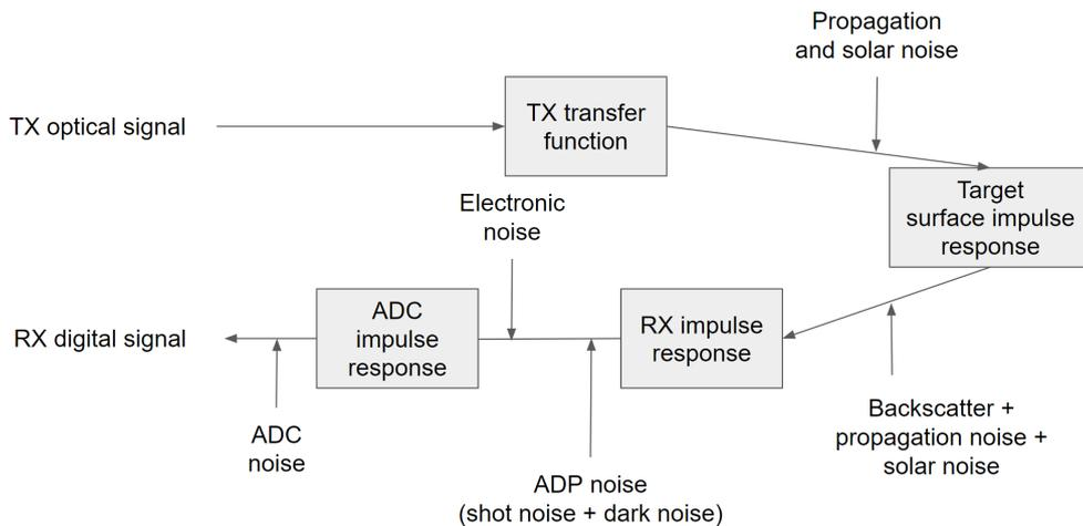
**Figure 4.1:** Simplified block diagram of an estimation of what affects the laser rangefinder signal throughout transmitting and receiving. The blocks represent convolution with the signal, while the arrows are addition to the signal.
