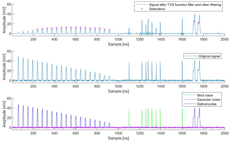
**Figure 5.8:** A signal after using the linear TVG function filter, the original signal and its different segments.
