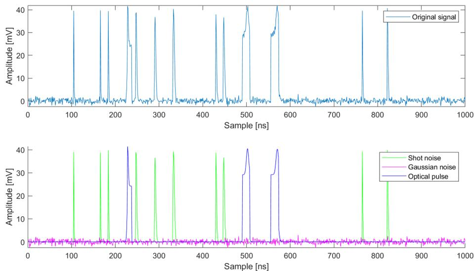
**Figure 4.2:** Simulated original signal and its different segments.
