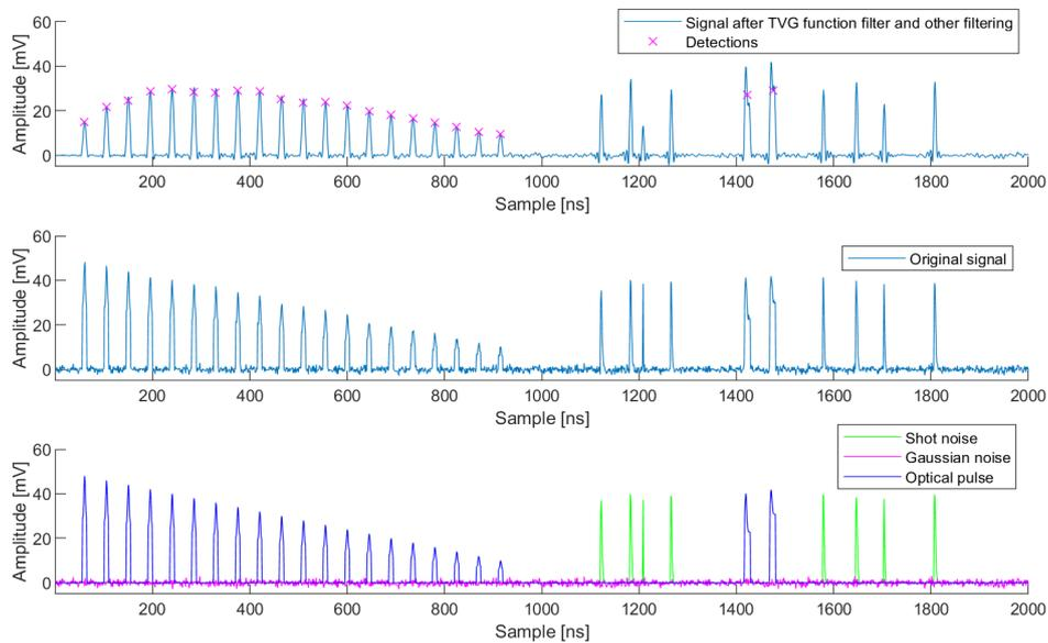
**Figure 5.10:** A signal after using the inverse exponential TVG function filter, the original signal and its different segments.
