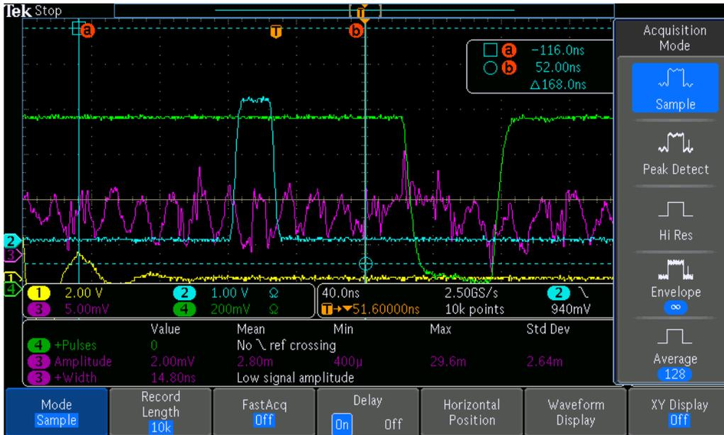
Figure 3.2: Oscilloscope view of a detection for an optical pulse.
