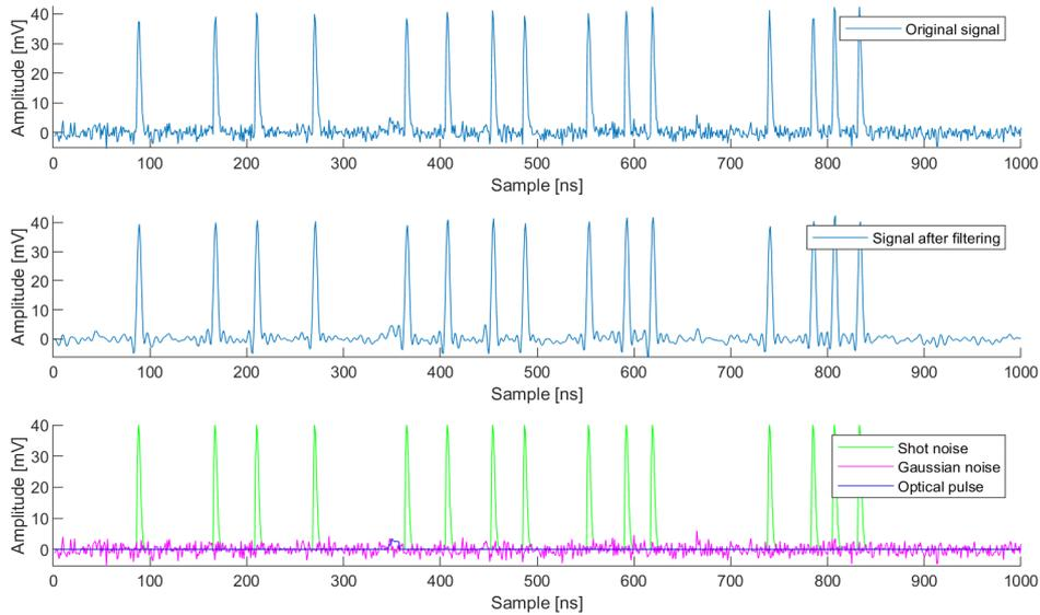
**Figure 5.6:** A signal when the detection method is failing to detect the optical pulse for case 3, the signal after filtering and its different segments.
