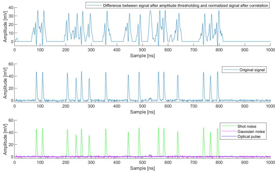
**Figure B.4:** Signal after calculating the difference between the signal after amplitude thresholding and after correlation, original signal, as well as its different segments.
