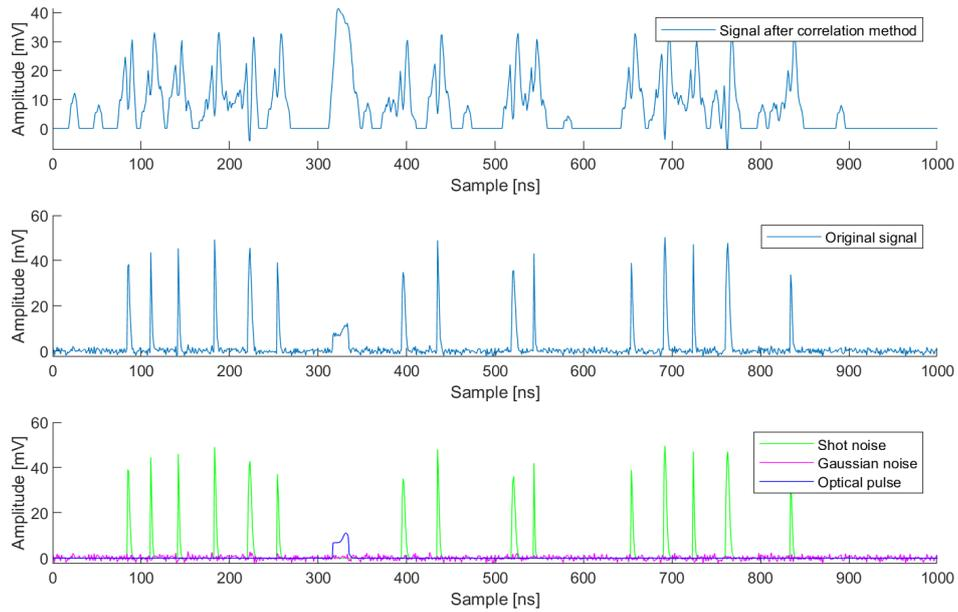
**Figure B.5:** The signal after correlation method, the original signal and signal segments for test case 5.
