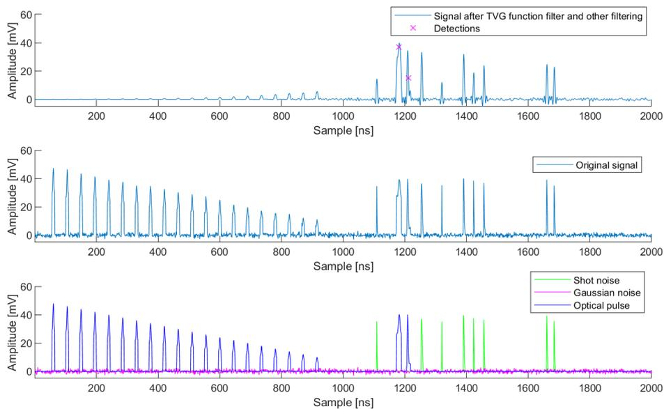
**Figure 5.11:** A signal after using the exponential TVG function filter, the original signal and its different segments.
