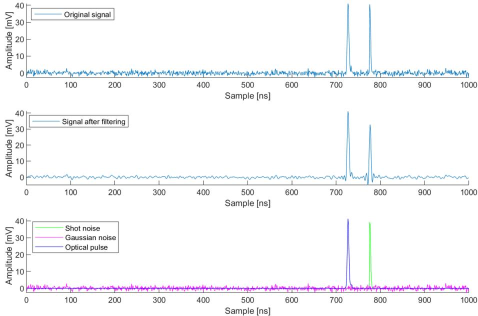
**Figure 5.5:** A signal when the detection method is failing to detect the optical pulse for case 1, the signal after filtering and its different segments.
