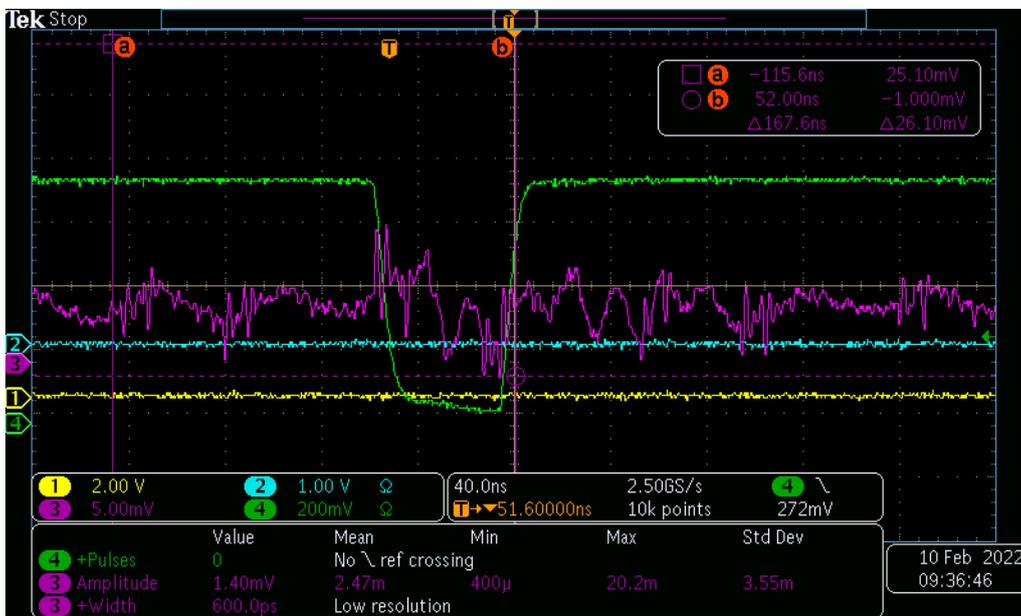
Figure 3.3: Oscilloscope view of a detection for a shot noise pulse, i.e. a false alarm.
