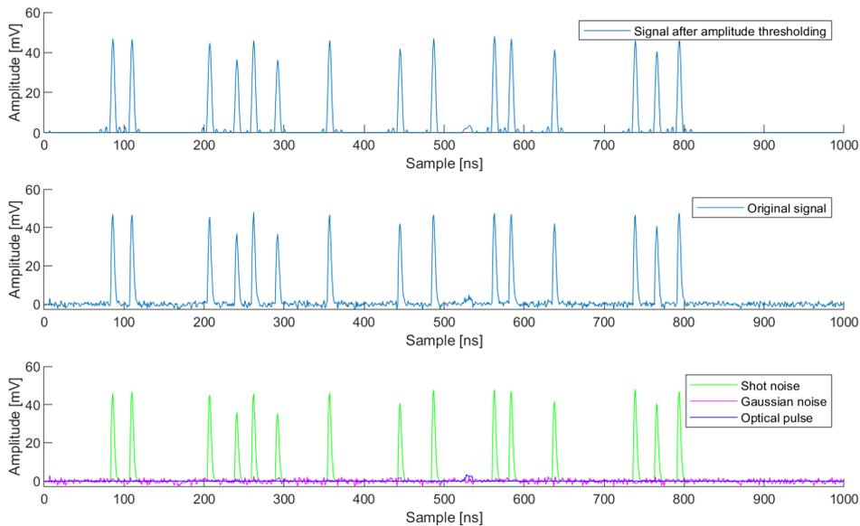
**Figure B.1:** Signal after amplitude thresholding, original signal and its different segments.
