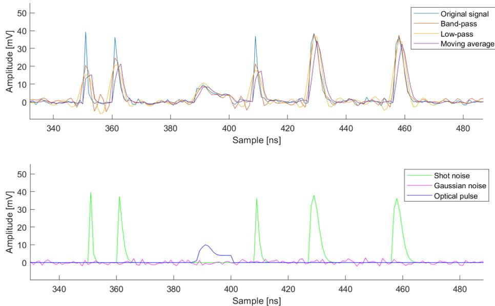
**Figure A.1:** Original signal and the signal filtered with different filters, as well as its different segments.
