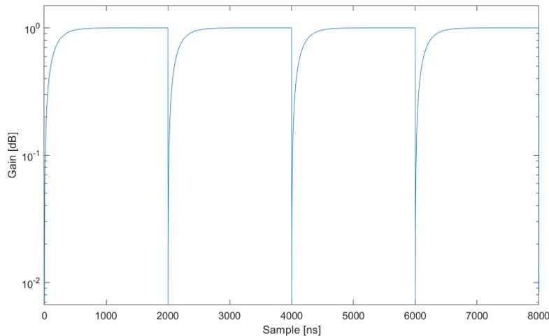
**Figure 2.2:** Ideal example of an analog TVG filter over four measurements. Amplitude and frequency are not true to reality, it is only to illustrate the principle.
