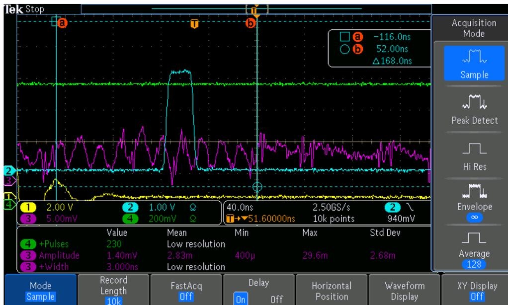
Figure 3.1: Oscilloscope view when there is no detection.
