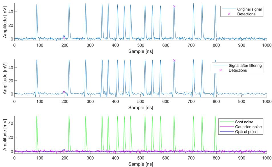
**Figure 5.7:** A signal when the detection method is failing (since a shot noise pulse is detected) for case 4, the signal after filtering and its different segments.
