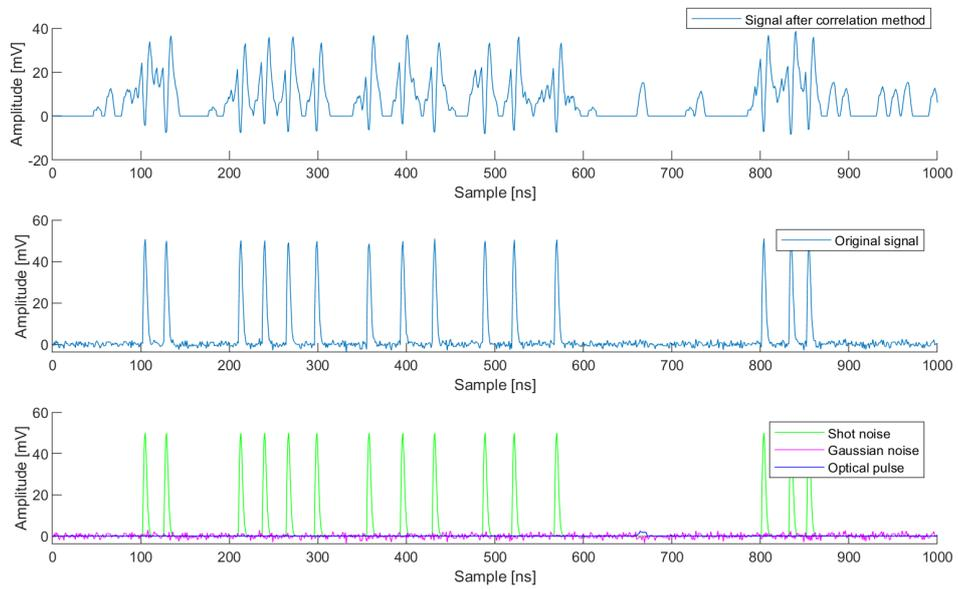
**Figure B.6:** The signal after correlation method, the original signal and signal segments for test case 6.
