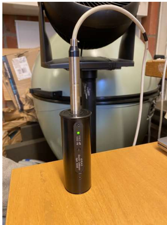
Figure 3.1: The figure shows a G.R.A.S 42AB, the black cylinder on the table was the speaker chamber producing 114 dB SPL at 1000 Hz and the grey part was the RM. The value the RM obtains in the chamber was used in the calibrations.
