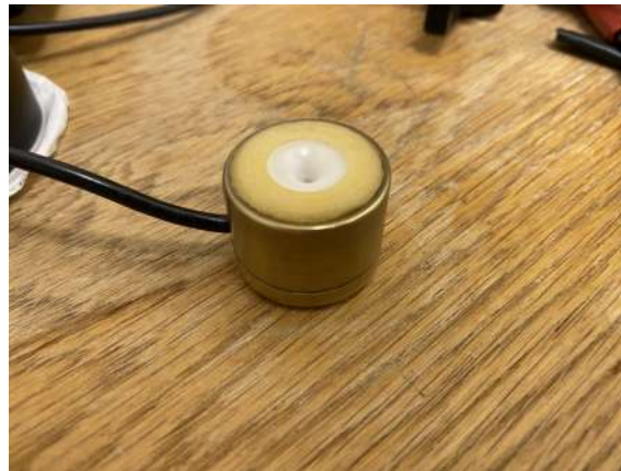
Figure 2.6: The SM that is used in the study can be seen in the figure. The microphone is inside a brass casing with yellow and white foam and a hole for the microphone [16]. This construction improves the sound insulation for the microphone [16].
