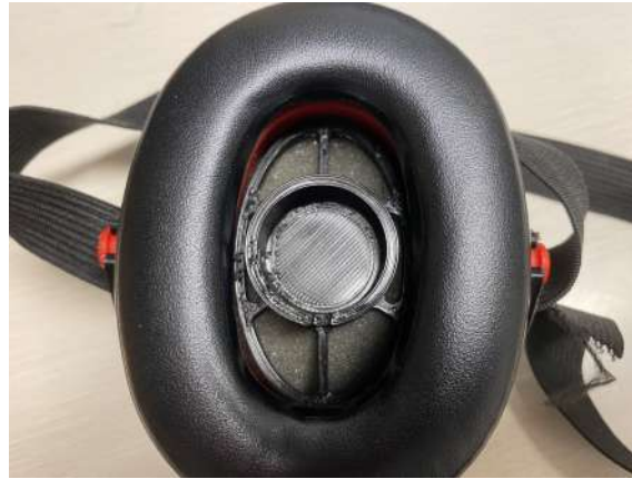
Figure 3.10: Final construction of the earmuff. The softband goes inside and under the attaching arrangement to apply pressure to the SM to get a clean connection between the SM and the skin. The softband can be adjusted with a clip.
