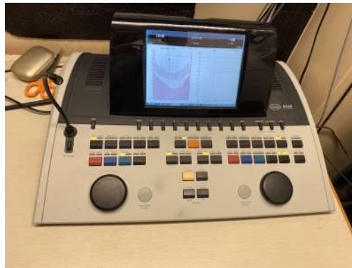
Figure 3.4: The audiometer AC40 (Interacoustics A/S, Assens, Denmark) used to simulate signals in all the trials. The audiometer could simulate different frequencies and dB HL levels for the B81 transducer and speaker inside the insulated room.
