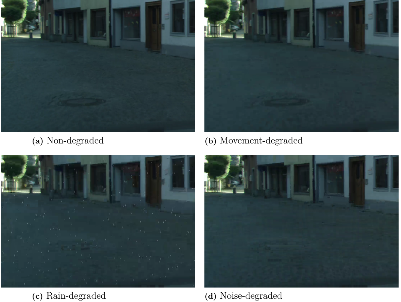
Figure B.4: Cropped image examples of video compression artefacts using lib264.
