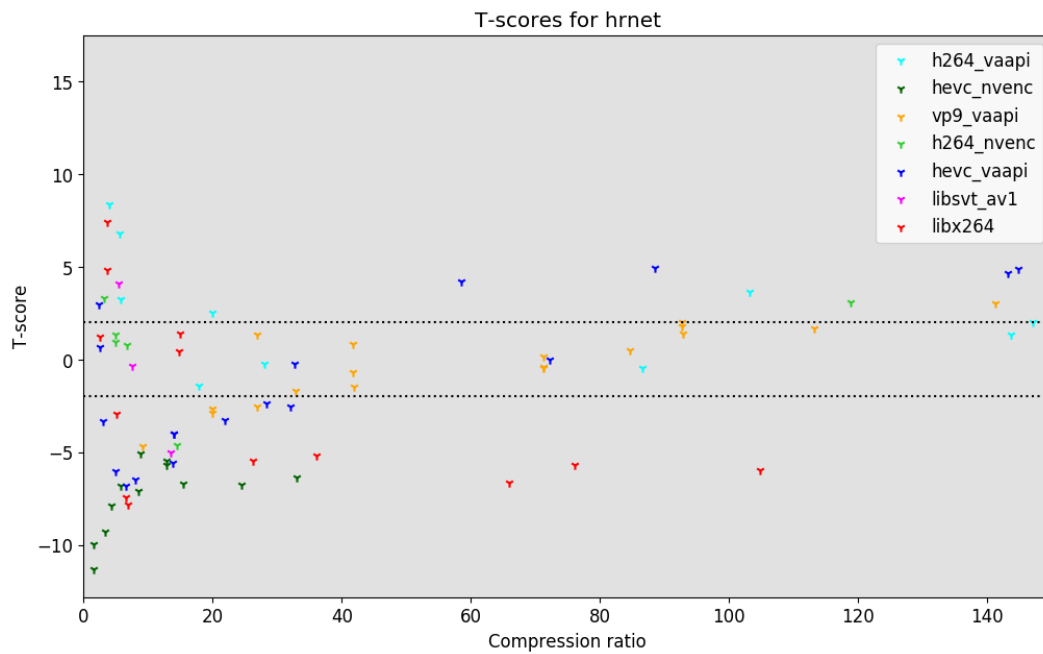
Figure 4.17: Plots of T-scores for the HRNet sweet spot candidates compressing the noise-degraded dataset.
