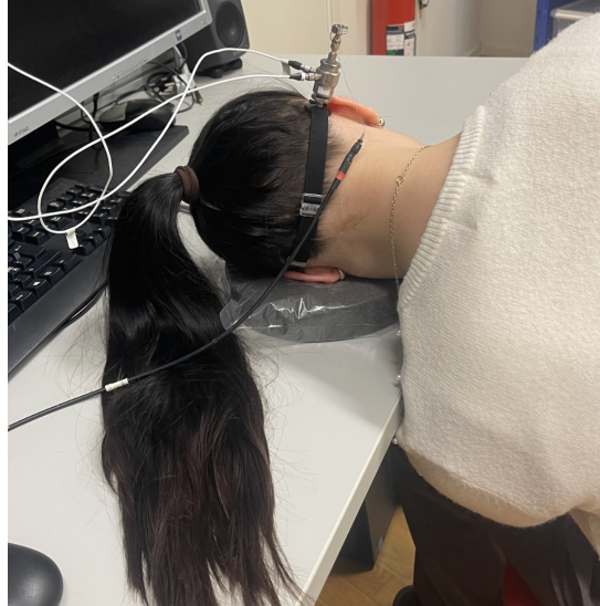
Figure 22: Mechanical point impedance measurement setup for data collection on test persons.
