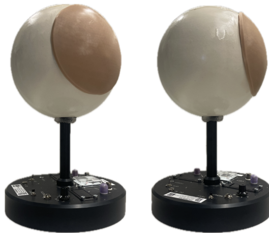
Figure 38: The new molded Ecoflex0010 scalp, 4 mm thick, on a HeadSim1.
