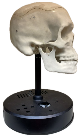
Figure 10: Cochlear's Head Simulator, model HeadSim 3D.
