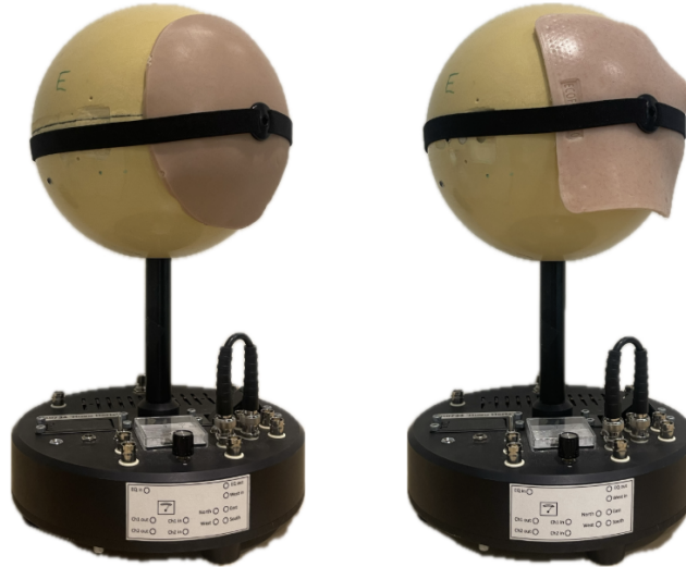
Figure 41: Side-by-side comparison of the new molded Ecoflex0010 scalp (left) and the old existing Ecoflex0010 (right).
