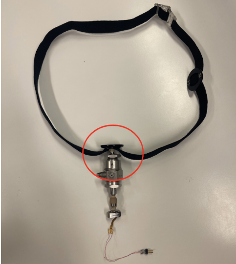
Figure 27: The Softband setup used in all measurements, using the snap of the Softband as an interface between the impedance head and scalp.
