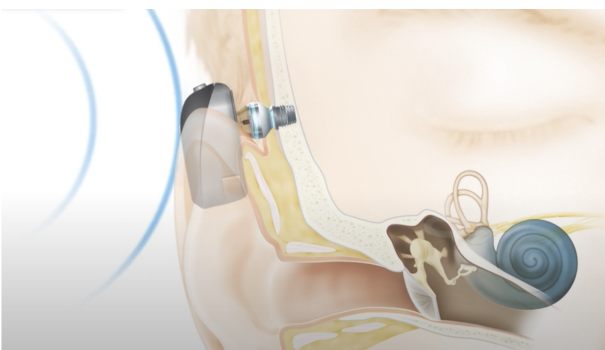
Figure 1: An illustration of the Baha connect system [6].
