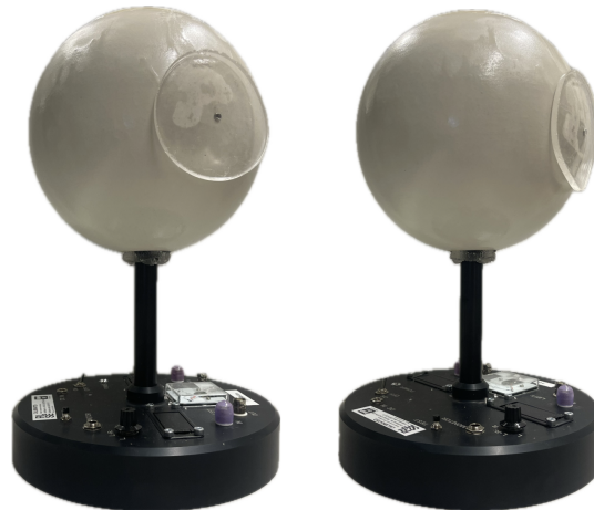
Figure 35: The crafted silicone scalp with 10% hard silicone & 90% soft silicone, 4 mm thick, on a HeadSim1.
