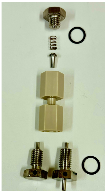
Figure 4.2: The tomography cell parts, comprising (from top to bottom), stainless steel top screw, spring, stainless steel top pin, PEEK cell house and two variants of the stainless steel bottom pin/screw. The variant to the right has an extension pin at the bottom, which was used for easier alignment during the nanoCT experiment. The two O-rings can be seen to the right, which are inserted between the steel screws and the PEEK cell to seal the cell house air-tight.
