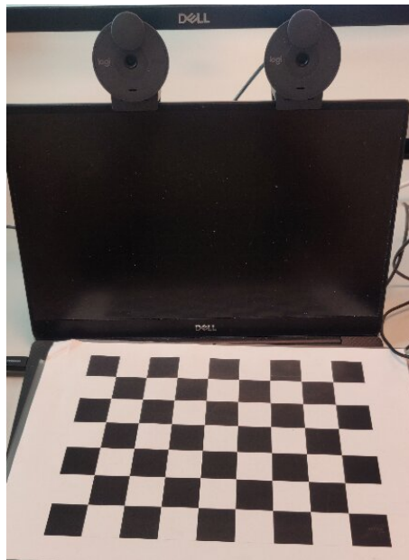
Figure 3.8: Setup of the stereo vision setup and the checkerboard for calibrating.
