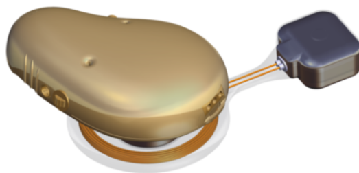
Figure 2.12: Active transcutaneous BCI with its implantation and external units. [8]
