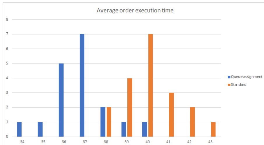
Figure 4.5: Average number of seconds to complete an order in system C. The system is running 8 AGVs, and performing 50 orders per test. The mean time to complete an order is 36.8 s for our queue assignment algorithm and 40.1 s for Kollmorgen’s standard algorithm. This is 9.0% increase in throughput for the system using our queue assignment.
