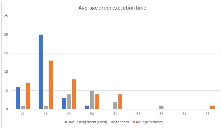
Figure 4.3: System B with five vehicles running. Queue assignment has a mean of 48.0 seconds, standard has a mean of 49.7 seconds, and MV has a mean of 48.8 seconds. This puts our solution at 3.5% higher throughput than the standard, and 1.6% higher throughput than MV. These numbers are summarized in Table 4.2
