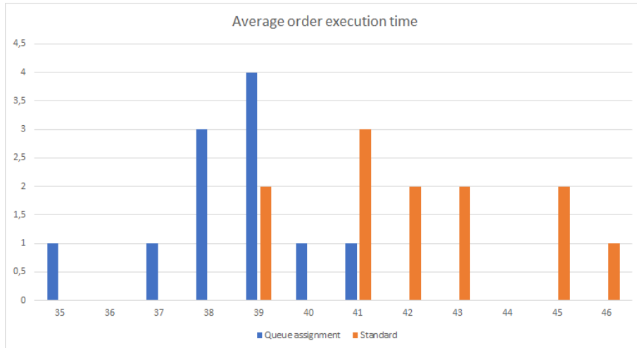
Figure 4.6: Average number of seconds to complete an order in system C. The system is running 10 AGVs, and performing 50 orders per test. The mean time to complete an order is 38.5 s for our queue assignment algorithm and 42.25 s for Kollmorgen’s standard algorithm. This is 9.7% increase in throughput for the system using our queue assignment.
