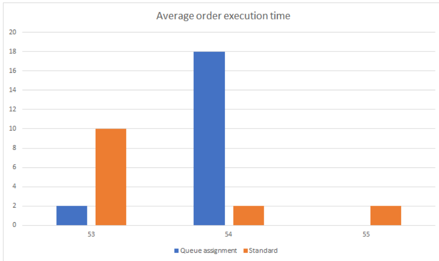
Figure 4.1: Histogram showing the average time in seconds to complete an order in system A running 2 vehicles. Each data point is an average of 50 orders. More details can be found in in Table 4.1
