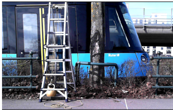
Figure 3.11: SL18 tram at Grefsen with the falling weight set up.
