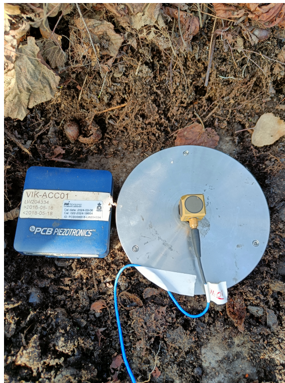
Figure 3.2: Sensor, mounted on top of a metal foundation at Grefsen.
