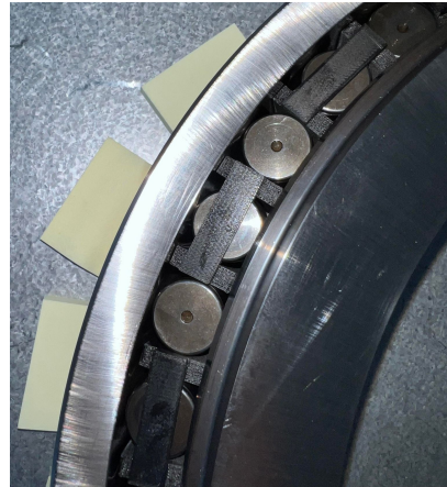
(a) The SAT prototype bearing with the segments assembled in it (b) Close-up of segments and rollers in the SAT prototype bearing
