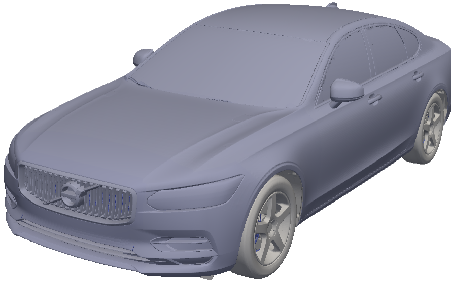
Figure 4.1: Example stl model. The car is built up with almost 4 million triangle surfaces. Model courtesy of Volvo Cars.
