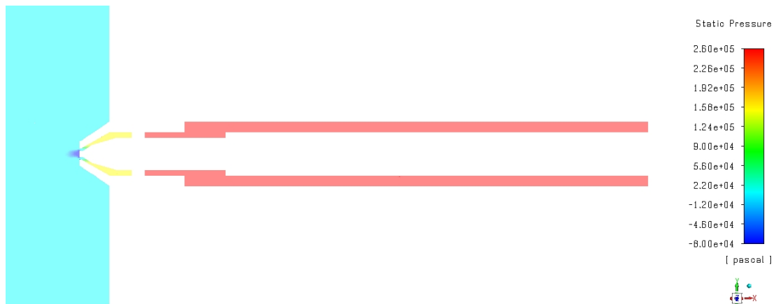
(a) Pressure contour plot shown on a sectional plane of the atomizer
