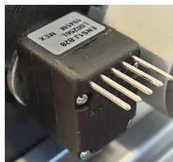
Figure 4.6: The rotary encoder used for the prototype, Bourns ENS1J-B28-L00256L - 256 CPR 5V 3000rpm.
