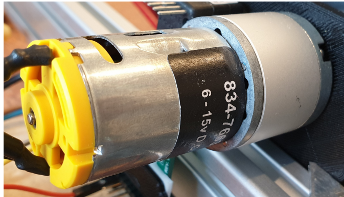
Figure 4.5: RS PRO - Brushed DC Geared Motor, Output Speed 366 RPM, 12 V dc.
